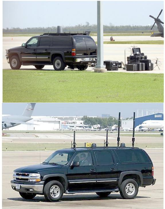
only a few VHF antennas. They have sometimes been seen carrying a single, large satellite antenna "hump" on the roof, while others carry two smaller satellite antenna radomes. One of the more prominent features that some of the presidential vehicles often carry are pairs of large, thick, black vertical antennas that seem to have either rubberized "boots" or perhaps heat sinks at the base.
