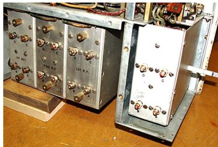
*Bandswitch shaft (shown partly withdrawn at right) must be pulled out all the way before the three front end cans (at left) can be removed.*
