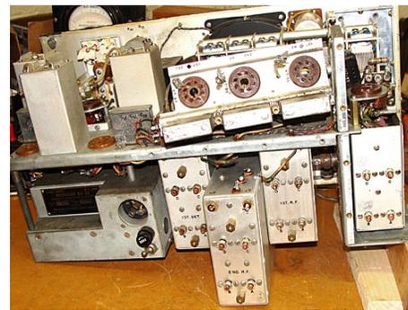
*One side of chassis was raised to obtain clearance for dropping out 2nd r.f. can. Note that tube shelf above cans has been tipped up to get access to wiring connections and mounting screws.*
