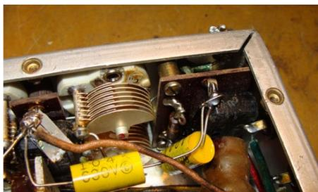
The new 0.1 uf capacitors (light-colored tubular units) installed in the 2nd r.f. can.
