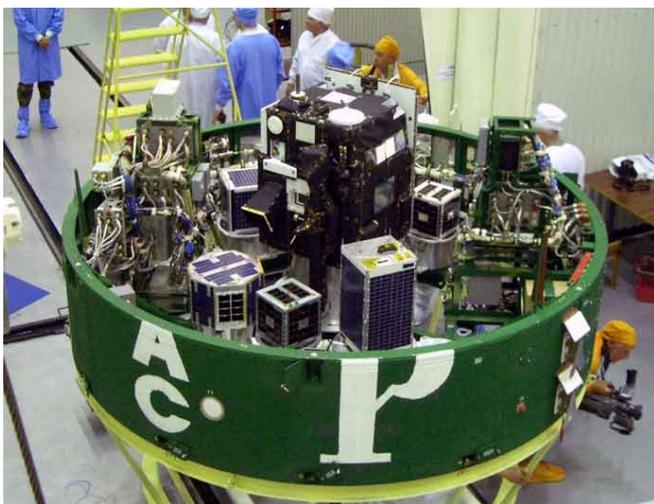
**Numerous other satellite passengers dwarf AO-51, shown here sitting in its upper stage carrying structure just prior to launch from the Baikonour Launch Complex in Kazakhstan. AO-51 is the small cube-shaped satellite shown in the lower left of the photo between the octagonal-shaped Italian UniSat-3 and the taller SaudiSat 2. (AMSAT Photo)**
