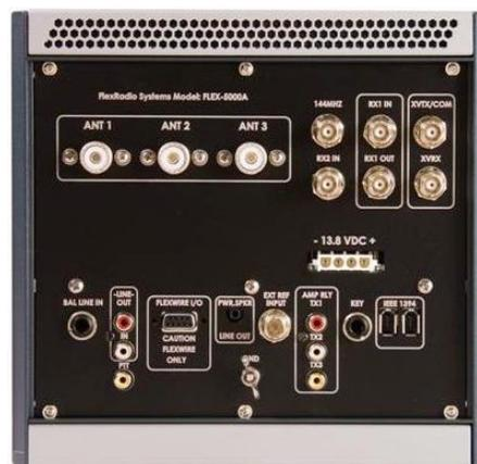
Figure 2C – Rear-panel view of the new FLEX-5000A full duplex 160M through 6M 100W all mode transceiver (Courtesy [www.flex-radio.com](http://www.flex-radio.com))
