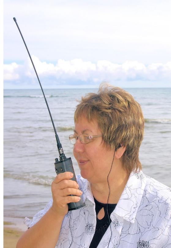
*Author's wife Kate Baker (KB1OGF/VA3OGF) makes a contact through the AO-51 satellite on the shores of Lake Huron in Michigan with her Kenwood TH-78A dual band HT. The extended "rubber duck" (MFJ Model 1717 from MFJ Enterprises) antenna and about 5 watts of uplink power provides just enough gain on the uplink and downlink to successfully work the satellite on near overhead passes. (KB1SF Photo)*
