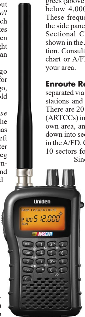
Popular Uniden BC72X-LT ($95) hand-held scanner with removable antenna covers many bands including the air band from 108-136.9875 MHz. (Courtesy: Communications Electronics, Inc.)
