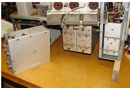
Here the last front-end can is buttoned up and ready to reinstall in its slot. The front-end tube shelf, above, has been dismantled and tilted aside to access the can connections. Note the three rectangular metal-cased capacitors.
