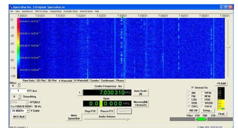
Figure 4. A "vertical waterfall" view. This is a 50 kHz slice of the 40M amateur CW band. Several CW stations can be seen, and the Morse characters along the side are time stamps.
