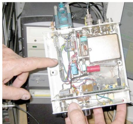
*This Global Positioning Satellite (GPS) receiver provides the time base for all his test equipment.*
