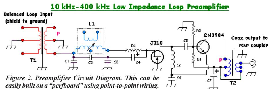
Figure 2. Preamplifier Circuit Diagram. This can be easily built on a "perfboard" using point-to-point wiring. (Diagram courtesy of Steve McDonald, VE7SL)
