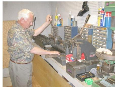
*Need a chassis or an angle bracket? It's a cinch when you have a professional hand brake.*
