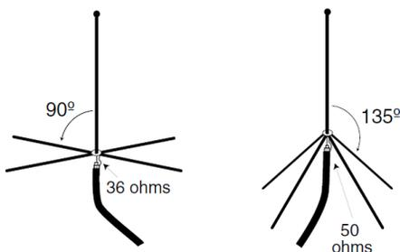
*The angle of the radialelements affect the feed point impedance of a ground plane vertical.*
