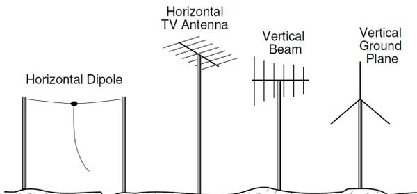
*The polarization of an antenna is simply its relationship to the surface of the earth.*
