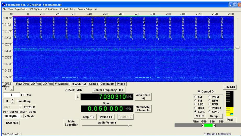
Figure 5. A “horizontal waterfall” view. This is the same slice of 40M as in Figure 4, but viewed horizontally.
