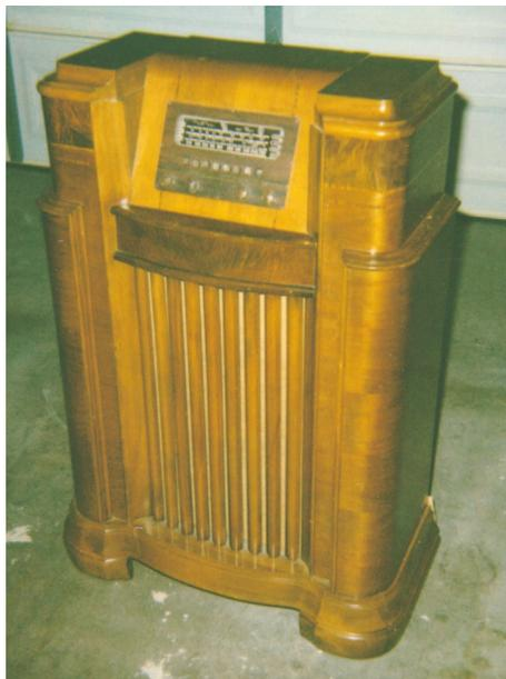
*A 1941 Philco model 41-285 the “McArthur Set”, as some call it. The original finish bleached, breached, and rubbed with oil by a well-meaning person. Knobs gone and es-cutcheon warped beyond help. Good starting material, though.*
