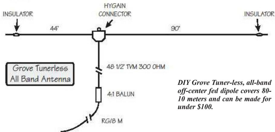
**DIY Grove Tuner-less, all-band off-center fed dipole covers 80-10 meters and can be made for under \$100.**
