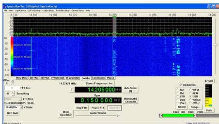
Figure 6. A combination spectrum analyzer and vertical waterfall view. This is a 50 kHz slice of the 20M amateur phone band. The spectral content of the voice is clearly visible. One can even tell whether the operator is using a microphone tailored for DX (more high frequency content) or ragchewing (more low frequency content).
