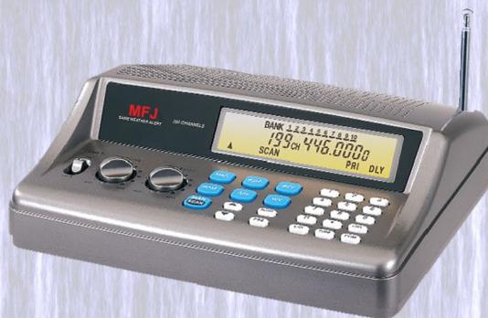
**Generous backlit LCD and 3" speaker. Front panel on/off switch with separate volume and squelch controls, 3.5mm headset jack for private listening. Includes pull-up BNC antenna and 120VAC to 9VDC adapter. Measures a compact 8 1/4" x 6 7/8" x 2 3/8" inches and weighs just 24.3 ounces.**
