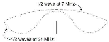
*A 67-foot dipole is half-wavelength at 7 MHz, but 1-1/2 wavelengths at 21 MHz. As the frequency increases, wavelength decreases.*
