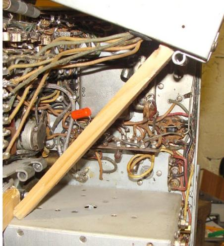
*BC-344 power supply has to be propped out of the way to get at lower i.f. adjustments.*
