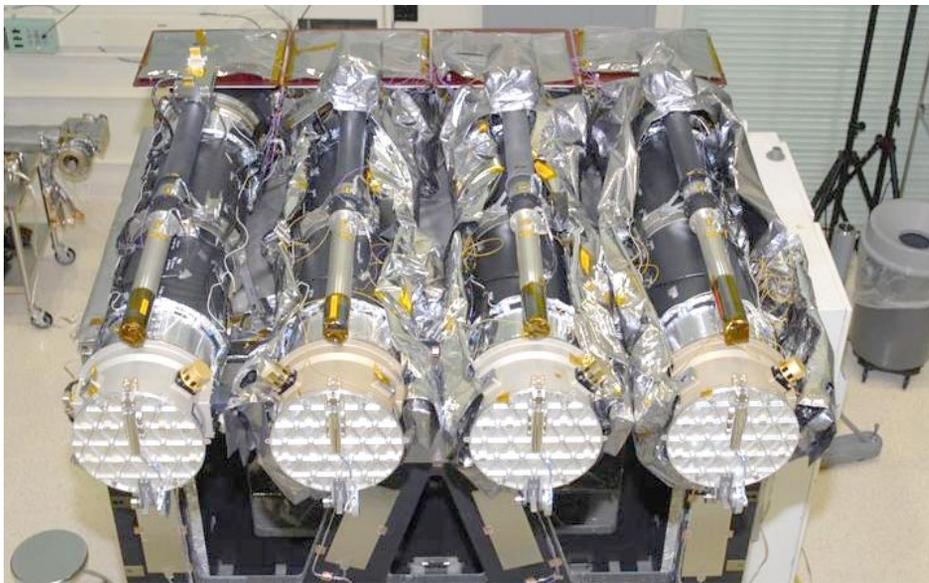
Main Atmospheric Imaging Assembly (AIA) installed in SDO (Courtesy: NASA/GSFC/AIA)
