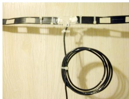
*The center of the folded dipole, wire-tied to the plexiglass "T", with solder joints sealed with silicone sealant. (Photo by author)*
