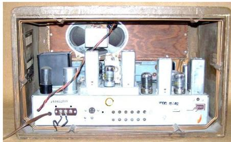
*Back view of 1948 Philco table radio. Note the loop antenna wound on the inner rear perimeter of the box. (Image copyright 2003-2010 Daryls Clocks Galore)*
