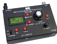
MFJ-9200 runs on any power source between 8 and 15 VDC and draws a miserly 40 mA on receive with the display backlight turned off – perfect for prolonged off-the-grid adventures.
