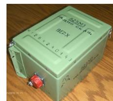
**This is the 28 Volt Orlan Spacesuit battery whose lack of a full charge precluded ARISSat-1's on-orbit test in April. Russian Space Agency officials assured AMSAT that this battery would once again be fully charged and inserted back into the spacecraft prior to ARISSat-1 being tossed overboard. (Courtesy: The ARISSat Team and Energia)**
