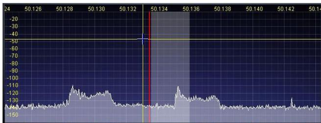
*Just like the good old days! As shown by the band scope on the FLEX-1500 SDR, during the 2011 June VHF QSO Party, 6-meters was alive and well. Here in Minnesota, K0DU (left, Colorado) and W4TP (right, Alabama) were booming in for hours on end. – NT0Z*
