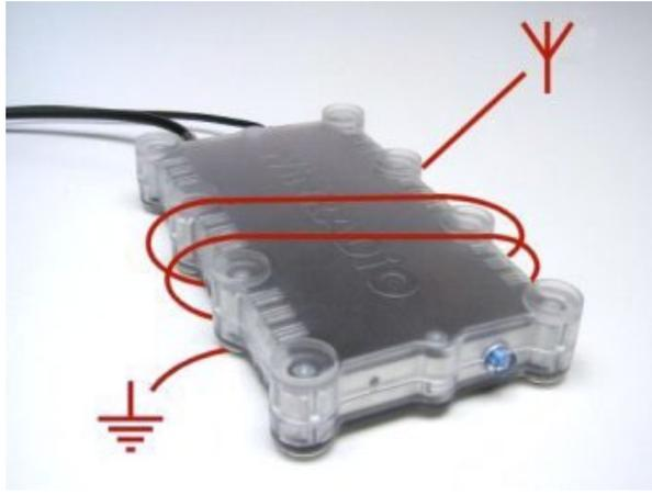
The WinRadio "active ferrite" antenna. (Courtesy WINRADIO Communications)
