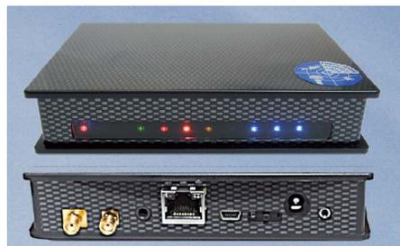
The audio output is via a 3.55mm stereo jack or it can be streamed over USB/Ethernet, and onto the Internet. The BaseStation software can also handle receiving ACARS digital signals using an audio port, but does require a separate ACARS decoder that is available as Freeware.
