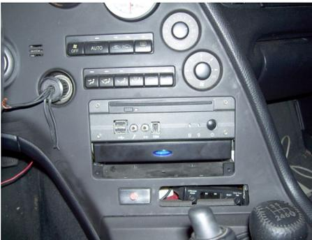
**Photo 4a (above) shows the in-dash PC mounted in the space formerly occupied by the AM/FM/CD player. The pop-out monitor is directly below the PC. Photo 4b (below) shows the monitor in its extended position, with Microsoft Windows XP on the display.**
