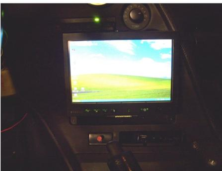
he used was to replace the control system with software that allowed the whole system to be tuned. To do this, he installed an in-dash PC that he bought from [www.mp3car.com](http://www.mp3car.com), one of several places from which you can buy PCs made for cars, as well as in-dash monitors, AM/FM receivers (to replace the functionality lost when you install a PC and/or a monitor in your dash), and more.
