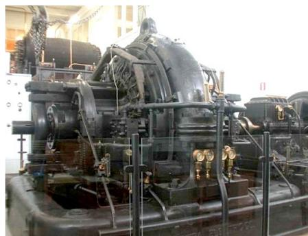
*SAQ, Grimeton, Sweden (17.2 kHz) uses a 1920s General Electric RF alternator to send its powerful CW signals (Source: Wikipedia; Author, Gunther Tschuch)*
