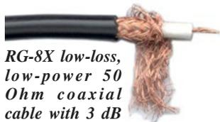
**RG-8X low-loss, low-power 50 Ohm coaxial cable with 3 dB attenuation per 100 feet at HF costs about 36 cents per foot in bulk. (Courtesy: Universal Radio)**
