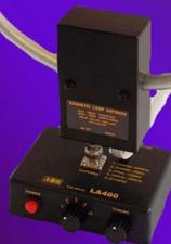
**Ultra-wide reception range** 10kHz ~ 500MHz. Four band selectable between 150kHz ~ 30MHz and precisely tunable for best receiving experience. Sharp alignment characteristics by electronic tuning. Exceptional 20dB gain thanks to built-in low noise amplifier.
