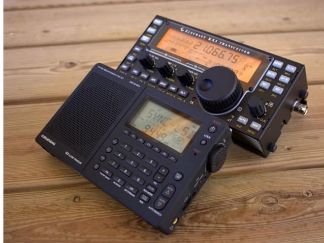
Natively decode (170 Hz) 60-WPM RTTY and display it right on the KX3’s VFO B display, which is alphanumeric.
