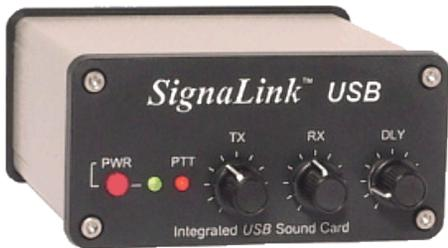
**Signalink USB interface (\$110) handles all modes and connects between your rig and computer. (Courtesy: Signalink)**
