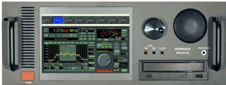
ing, and a re-writable CD-ROM or DVD drive makes archiving of recordings easy. The unit is capable of unattended operation and, if the client/server option is fitted, it can be operated remotely via a standard TCP/IP connection such as LAN or the Internet. The recorded audio can also be remotely searched and streamed to the operator.
