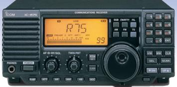
The Icom IC-R75A may be the best value today in a communications receiver. Has dual PBT, coverage to 60 MHz, notch and 99 alpha memories. Now includes UT-106 DSP.
