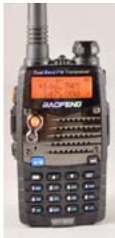
**Baofeng UV-5RA (\$35 online) features keypad and belt clip on radio, instead of battery pack. It meets new Part 90 requirements including narrow band capability and 2.5 kHz channel step—though these features are not required for amateur use.**
