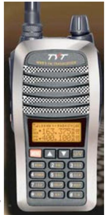
**TYT TH-UVF-1A (\$100) covers 2-meters/440 MHz with .5 to 4 watts transmit, 7.4V 1500 mAh Li-ion battery, drop-in charging base, AC adapter, SMA type antenna, belt clip and carrying strap. (Courtesy: Universal Radio)**
