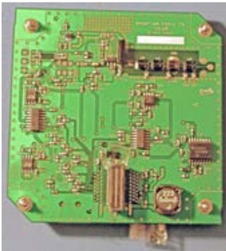
Engineering model of FOX-1A's 2-meter transmitter board. (Courtesy: AMSAT-NA)
