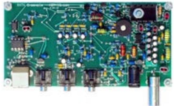
Softrock RX/TX Ensemble (Courtesy: Softrock SDR)
