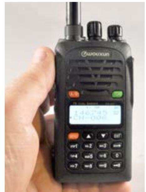
**Wouxon KG-UVD1P (\$110) features 5 watts VHF, 4 watts UHF, Li-ion battery, intelligent drop-in charger, flexible SMA-J (female) antenna and belt clip.**
