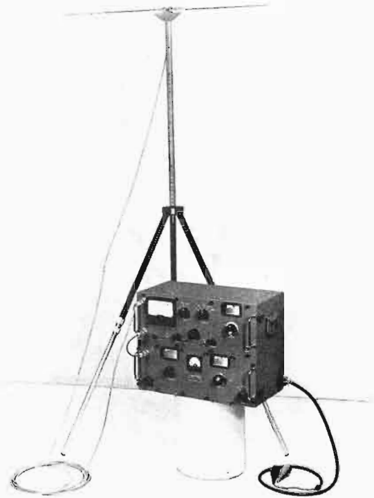
Fig. 5. A VHF field-strength meter of professional quality. (Courtesy of Nems-Clarke Company.)
