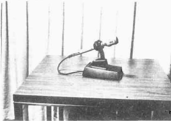
Fig. 38. Microphones without rubber isolation doughnuts can add this feature to mechanically isolate the microphone from the table as shown.
