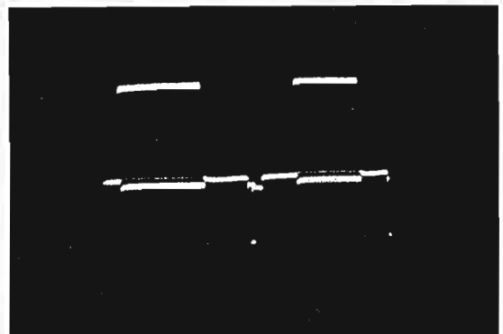
Fig. 77. Negative streaking—window signal—vertical.
