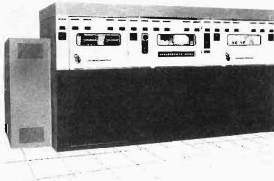
Fig. 1. Front view of the Continental 317C 50 kw Transmitter (Courtesy Continental Electronics Co.).
