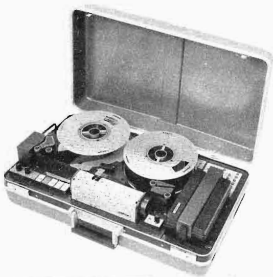
Fig. 102. VR-3000 portable quadruplex video tape recorder.
