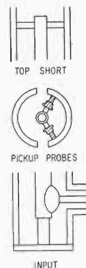
Fig. 49. Cross section of traveling-wave antenna at input, aperture, and top.
