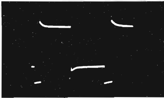
Fig. 69. Window signal—lows depressed, highs raised—horizontal.
