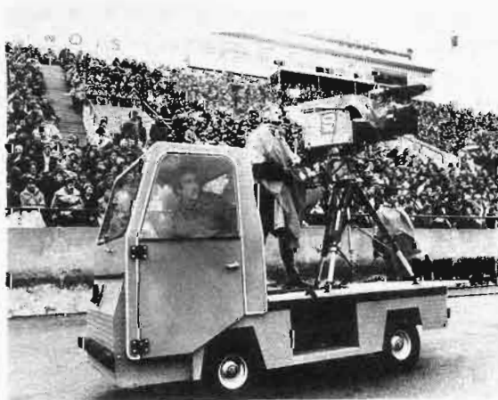
Fig. 34. Sideline camera on battery-operated mobile cart.
