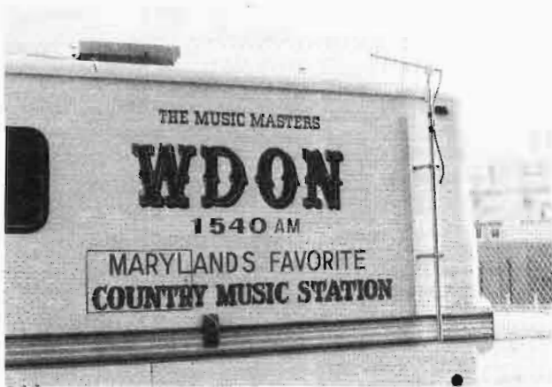
Fig. 5. The transmitting antenna is mounted to rotate 360 degrees and can be raised 10 ft. above the vehicle. The transmission line is attached to a reel inside the van to provide the additional length.
