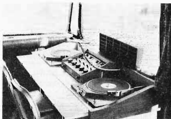
Fig. 2. A commercially available console was utilized with plug-in provisions for cartridge tape equipment. Two chairs are provided for side-by-side interviews.
