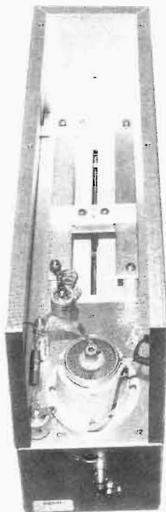
Fig. 31. Photograph of IPA anode tuning circuit.
