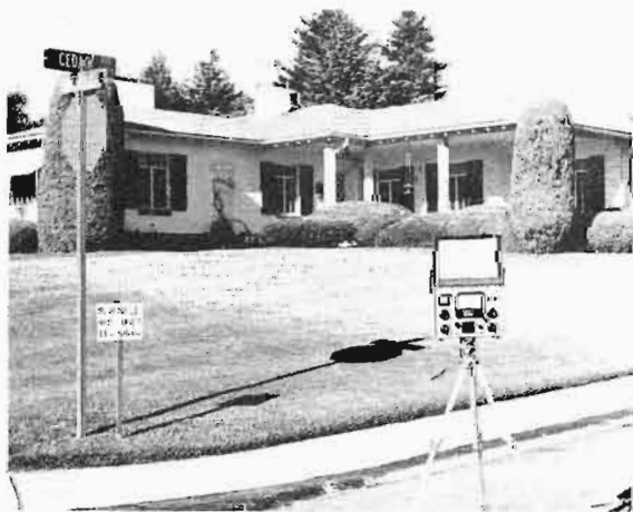
Fig. 7. Typical monitoring point location. Note freedom from overhead wires, underground cables, easily referenced location, etc.
