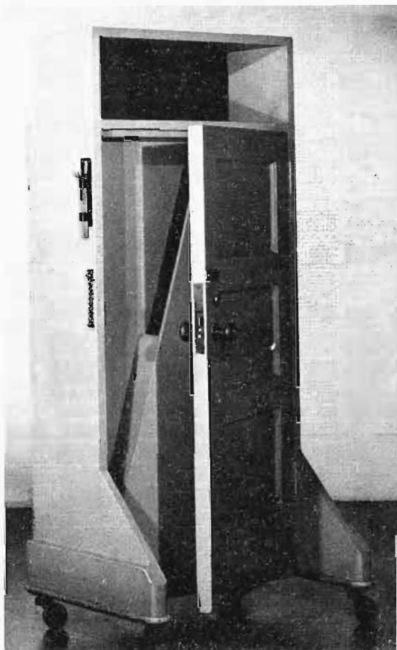
Fig. 50. Sound-effects door (front) showing door latch, chain, and acoustical chamber for resonance.
