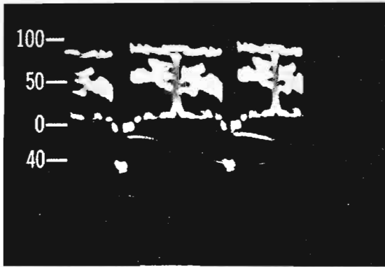
Fig. 62. Partial clamping failure—horizontal—(A-scope presentation expanded to normal height).
