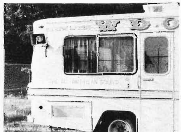
Fig. 7. Public address speaker is mounted on side of van and is capable of being rotated 180^\circ .
