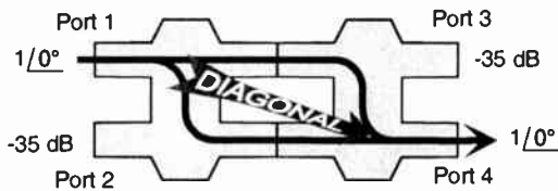
Figure 4.13-30. Hybrid ring, showing low-loss diagonal energy flow.
