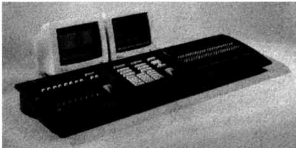
Figure 5.16-29. The most sophisticated consoles utilize dual CRT displays and can control very large quantities of dimmers with equal number of discrete channels.
