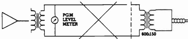
Figure 3.11-1. DON'T meter the signal across the input to the repeat coil (transformer at right) and DON'T feed the repeat coil directly from another transformer, if possible.
