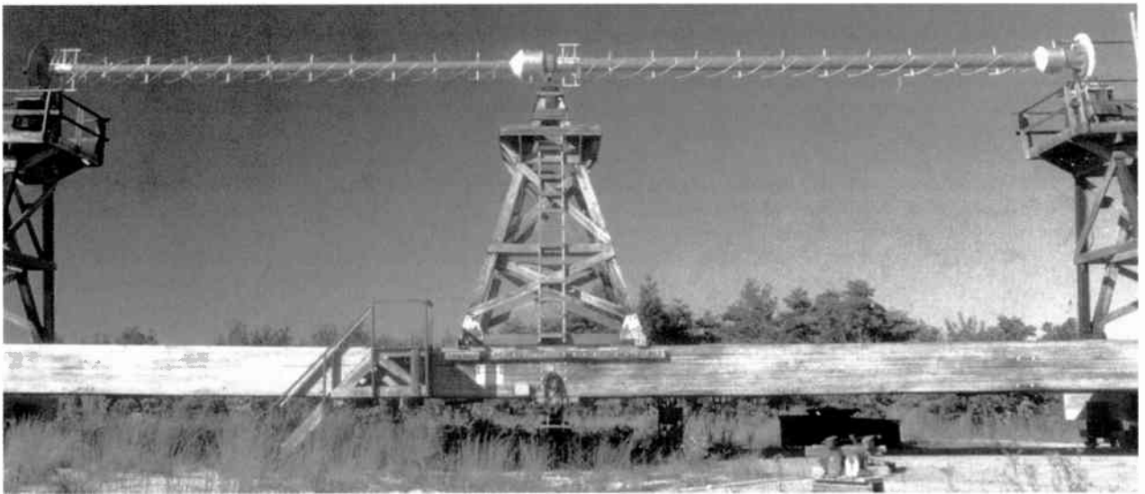
Figure 6.8-36. Spiral antenna on test range (Courtesy Dielectric).
