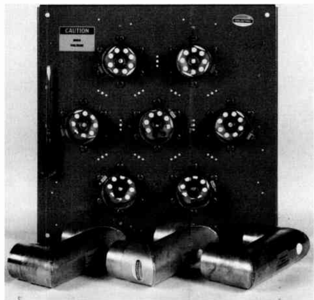
Figure 6.7-1. Seven-port patch panel.
