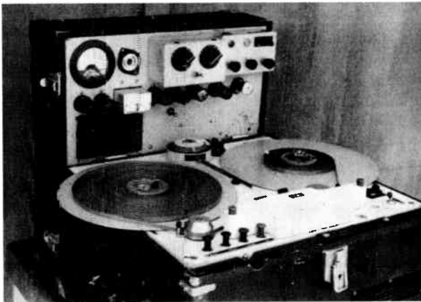
Figure 3.4-2. Early German Magnetophone brought to the USA after capture by officers in the U.S. Army Signal Corps. (From Jorgensen, The Complete Handbook of Magnetic Recording , 4th edition, 1995, McGraw-Hill. Reproduced with the permission of the McGraw-Hill Companies.)
