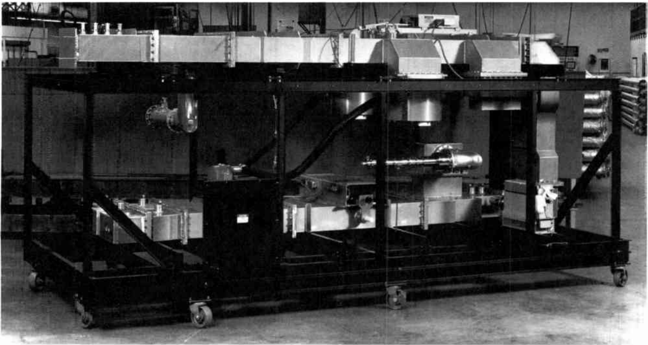
Figure 6.7-37. UHF 120 kW switchless diplexer.
