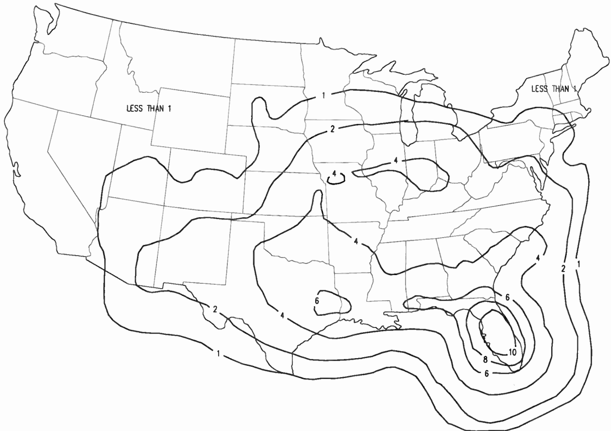
Figure 2.3-2. 1989–1993 Composite of measured lightning flash density per year. Flashes per square kilometer. (Data supplied by the National Lightning Detection Network.)
