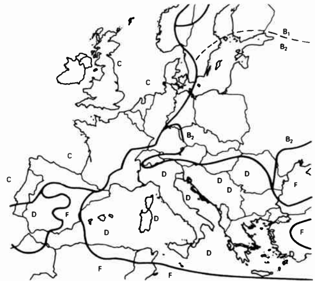
Figure 6.11-19. Rain rate climate regions for Europe. (From NASA Propagation Effects Handbook for Satellite System Design, ORI TR 1679.)
