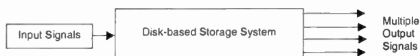
Figure 5.8-1. Simple application of a video server in a one in, many out configuration.
