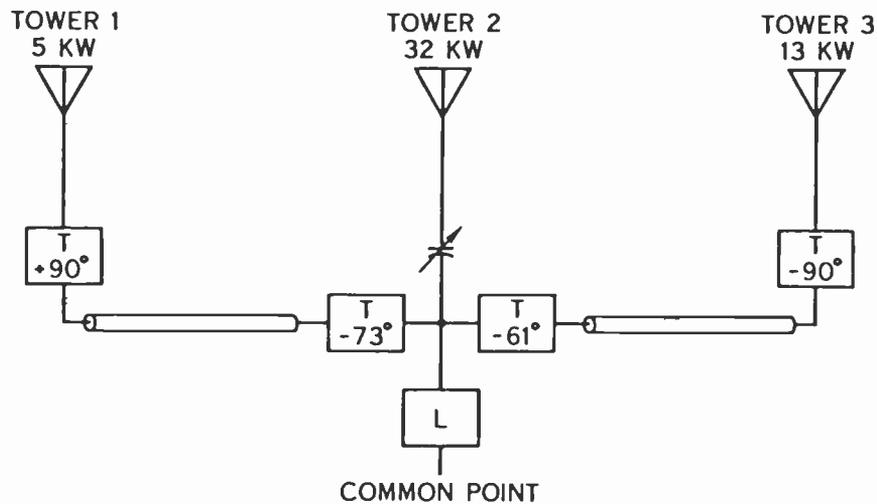
FIGURE 5. PHASOR WITH MINIMUM LOSSES
