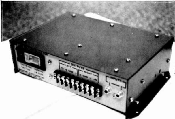
Broadcast Electronics EP-1 Phono Preamp shows extensive RF shielding to minimize both conducted and radiated interference.
