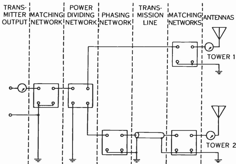
FIGURE 3. PHASOR BLOCK DIAGRAM
