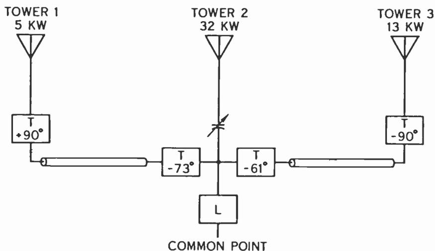
FIGURE 5. PHASOR WITH MINIMUM LOSSES
