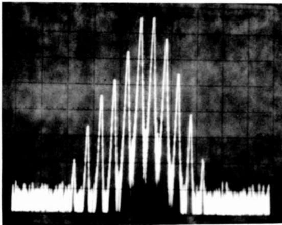
FIGURE 7. RF SPECTRUM OF AM SIGNAL INDICATING PRESENCE OF APPROX.  $20^{\circ}$  OF PEAK PHASE MODULATION. NOTE: THE 1dB REDUCTION IN APPARANT CARRIER AMPLITUDE AND 2nd ORDER SIDEBANDS ONLY 20dB BELOW DESIRED SIDEBANDS YET AM DISTORTION MEASURES 1%.
