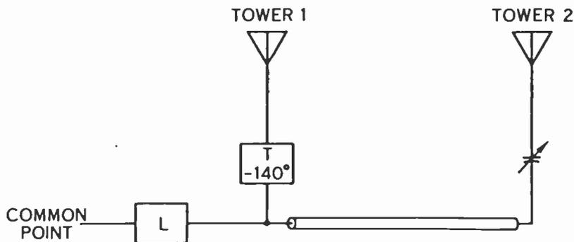
FIGURE 6. PHASOR WITH UNMATCHED TRANSMISSION LINE
