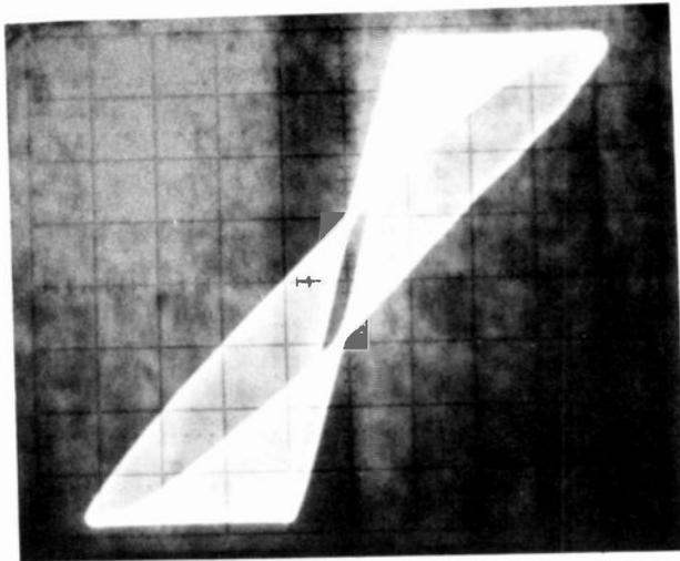
FIGURE 13. LISSAJOUS I.P.M. MEASUREMENT SHOWING  $8.6^\circ$  I.P.M. IN TROUGH AND  $13.1^\circ$  I.P.M. AT CREST OF MODULATION ENVELOPE (75% MODULATION DEPTH)
