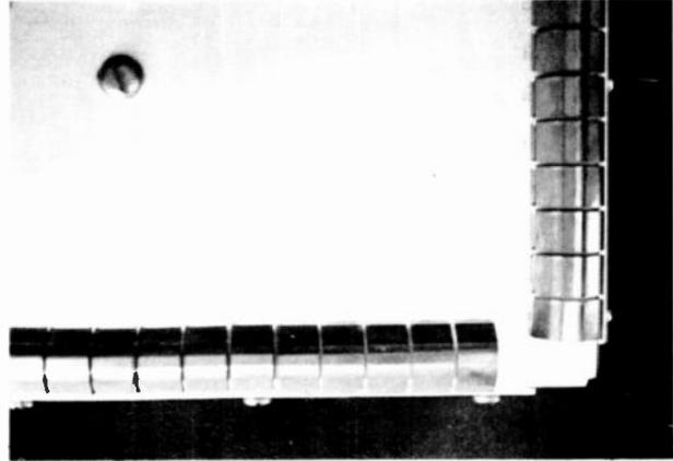
Figure 6 shows fingerstock used on the FM-30 transmitter to provide a positive RF connection between the door and the chassis.
