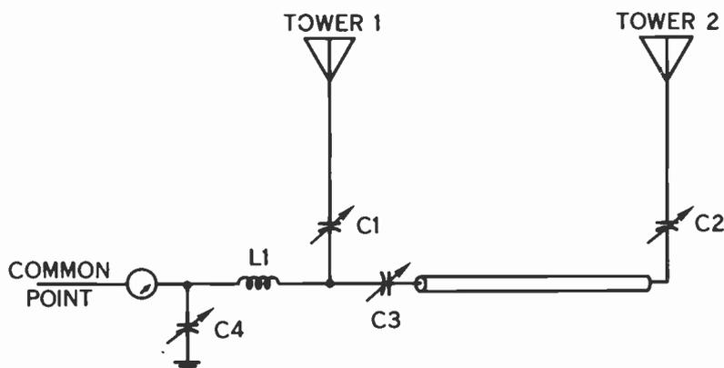
FIGURE 8. PHASOR WITH MINIMUM NUMBER OF COMPONENTS
