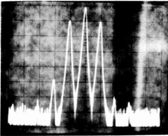
FIGURE 5. RF SPECTRUM OF ACTUAL AM SIGNAL INDICATING PRESENCE OF SMALL AMOUNT OF INCIDENTAL PHASE MODULATION. MEASURED AM DISTORTION OF 1%.
