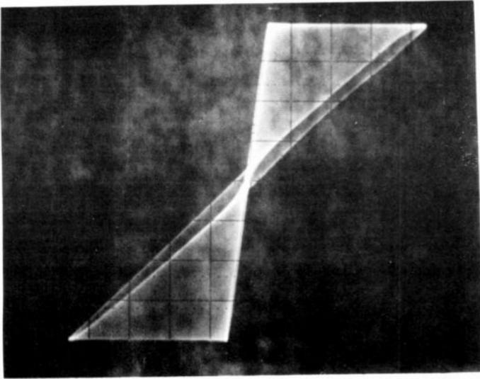
FIGURE 12. LISSAJOUS I.P.M. MEASUREMENT OF AM SIGNAL INDICATING APPROXIMATELY  $3.8^\circ$  PEAK PHASE DEVIATION AT MODULATION CREST. (80% MODULATION) AMPLITUDE OF TROUGH TOO SMALL TO MEASURE I.P.M.
