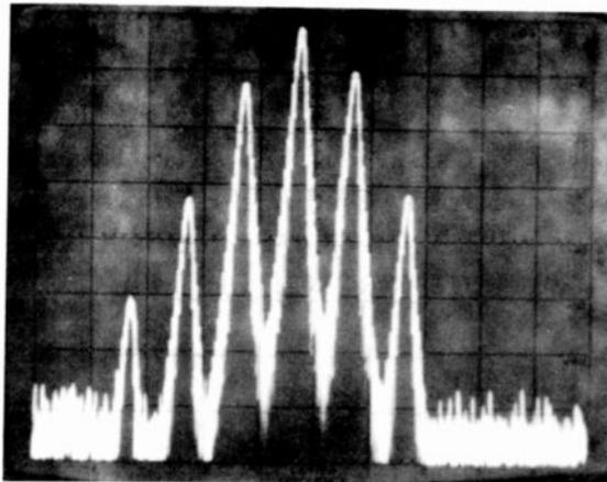
FIGURE 8. RF SPECTRUM OF AM SIGNAL INDICATING VERY EXCESSIVE I.P.M. OF APPROXIMATELY 1 RADIAN. NOTE: APPROX. 3dB REDUCTION IN APPARANT CARRIER AMPLITUDE (CARRIER SIGNAL IS HIGH SIGNAL ON THE LEFT) AND VERY HIGH ORDER AND UNBALANCED SIDEBAND PRODUCTS. YET AM DISTORTION MEASURES ONLY 1.5%.
