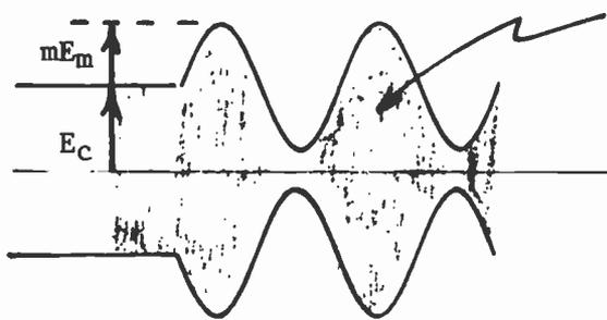
Carrier frequency and phase inside envelope is constant at  $\omega_c$  and independent of  $E_m$ .
