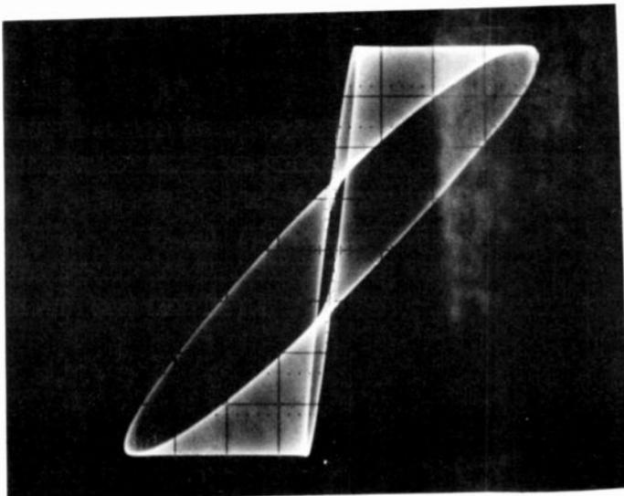
FIGURE 14. LISSAJOUS I.P.M. MEASUREMENT SHOWING  $8.6^\circ$  I.P.M. IN TROUGH AND  $17.8^\circ$  I.P.M. AT CREST OF MODULATION ENVELOPE (90% MODULATION DEPTH)
