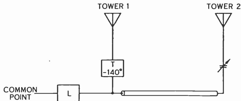
FIGURE 6. PHASOR WITH UNMATCHED TRANSMISSION LINE
