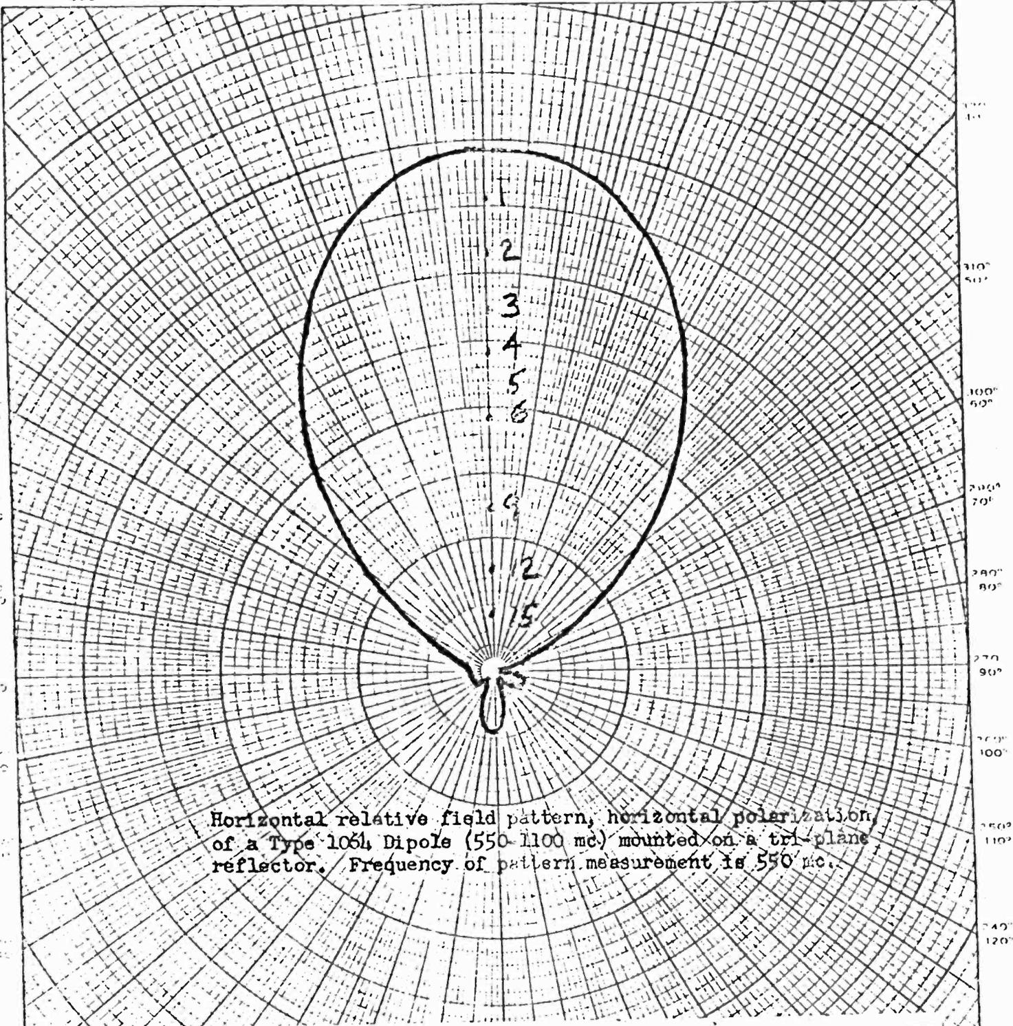
Horizontal relative field pattern, horizontal polarization,
