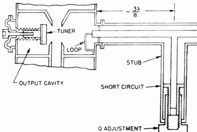
Figure 1. Schematic Diagram of Klystron Output Cavity and Variable Coupler Transformer
