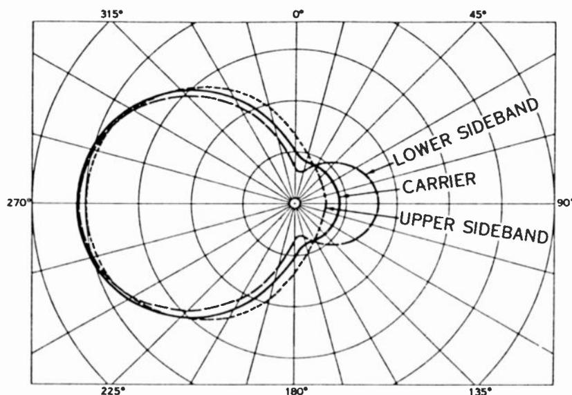
FIGURE 4. EXAMPLE OF POOR PATTERN BANDWIDTH
