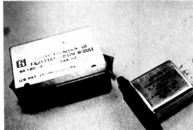
Figure 8 shows two commercial power line RF filters which provide good RF attenuation to VHF.
