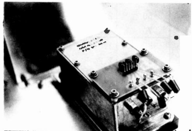
The modulated oscillator assembly in the FX-30 exciter has a "PI" section filter for each lead going into the unit. All leads finally pass through the feedthrough capacitor before entering the chassis.
