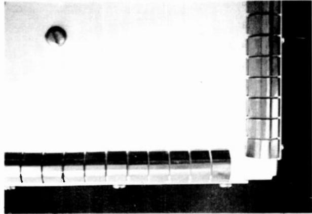
Figure 6 shows fingerstock used on the FM-30 transmitter to provide a positive RF connection between the door and the chassis.
