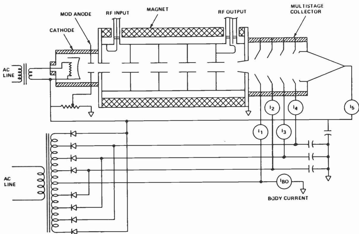
FIGURE 1. SIMPLIFIED SCHEMATIC FOR HIGH-EFFICIENCY, DEPRESSED-COLLECTOR-KLYSTRON UHF-TV FINAL AMPLIFIER
