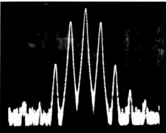
FIGURE 6. RF SPECTRUM OF AM SIGNAL INDICATING SIGNIFICANT I.P.M. NOTE: 2nd ORDER SIDEBANDS ONLY 30db BELOW 1st ORDER SIDEBANDS YET AM DISTORTIONS MEASURES 1%.
