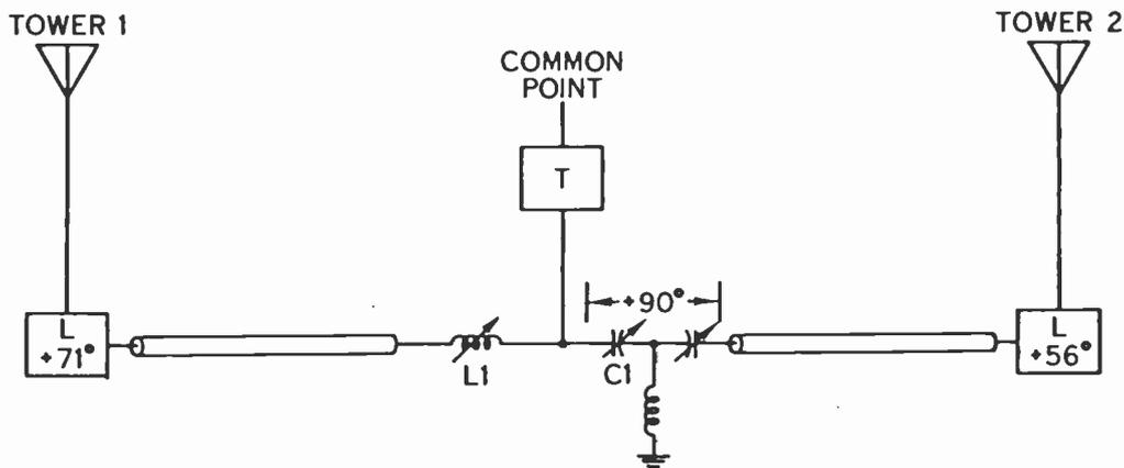
FIGURE 7. PHASOR WITH LEADING L NETWORKS AT TOWERS AND BACK-TO-BACK PHASE AND RATIO CONTROL
