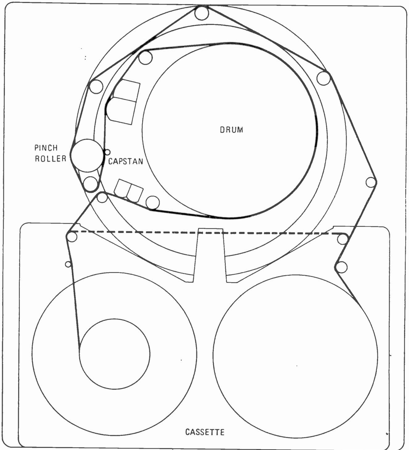
Fig. 1. RELATIONSHIP OF CASSETTE, DRUM, LOADING MECHANISM AND THE SIZE OF VTR MECHANISM
