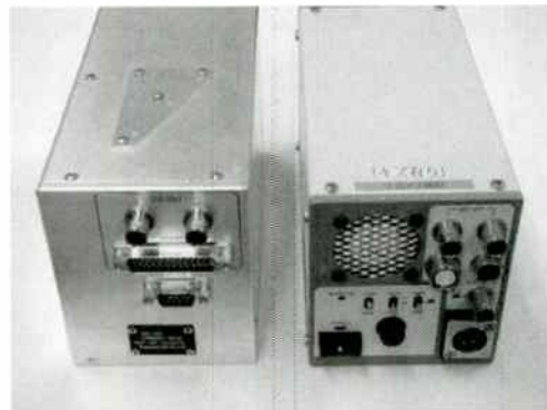
Fig.7 The compact HDTV camera modified for HDTV system (left) and the normal camera (right)
