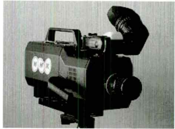
Fig. 9 300,000-pixel ultrahigh-speed, high-sensitivity portable color camera
