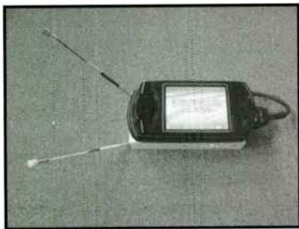
Figure 1 Emergency warning broadcast activation flag receiver
