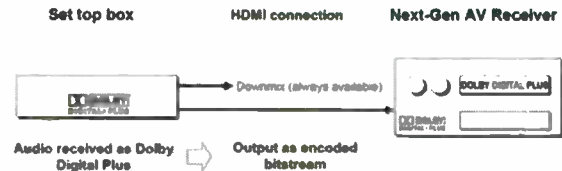
Figure 7: Scenario 3: Broadcast receiver device decoder-converter: Enhanced AC-3 input signal, HDMI connection (mixed or unmixed)
