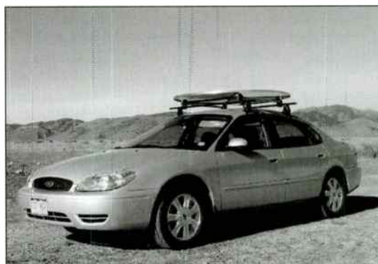
Figure 8- Ground plane antenna atop a test vehicle
