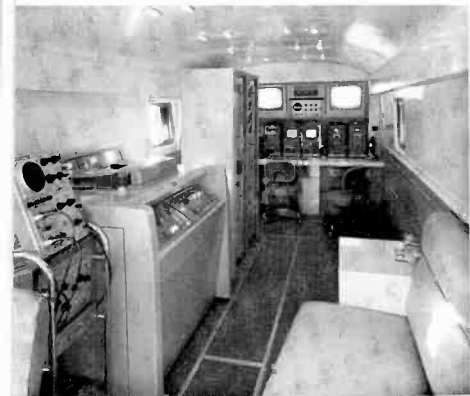
Ampex Videotape* Cruiser contains recorder, two camera chains, control and maintenance facilities and power generating equipment.
