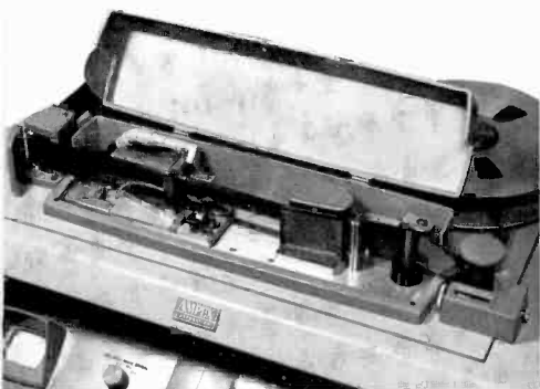
Erase head mounts at left of VR-1000 tape transport mechanism, Tape Timer at right. Installation is fast and easy; each unit replaces a tape idler.
