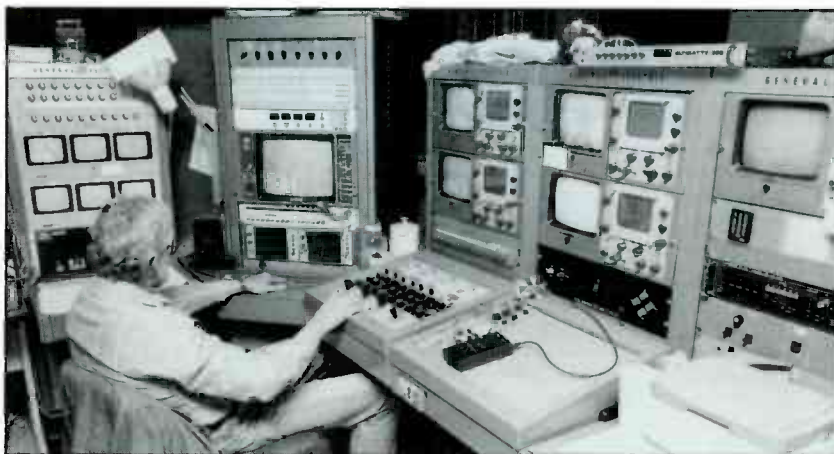
Master Control is where all broadcast signals are routed before they are sent to the transmitter and equipment is monitored for any potential problems that would cause the station to go off the air.
