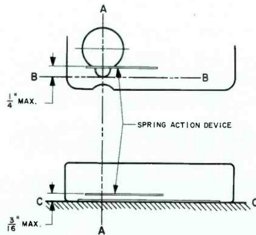
FIG. 1 REQUIRED SPRING ACTION DEVICE LIMITATIONS
