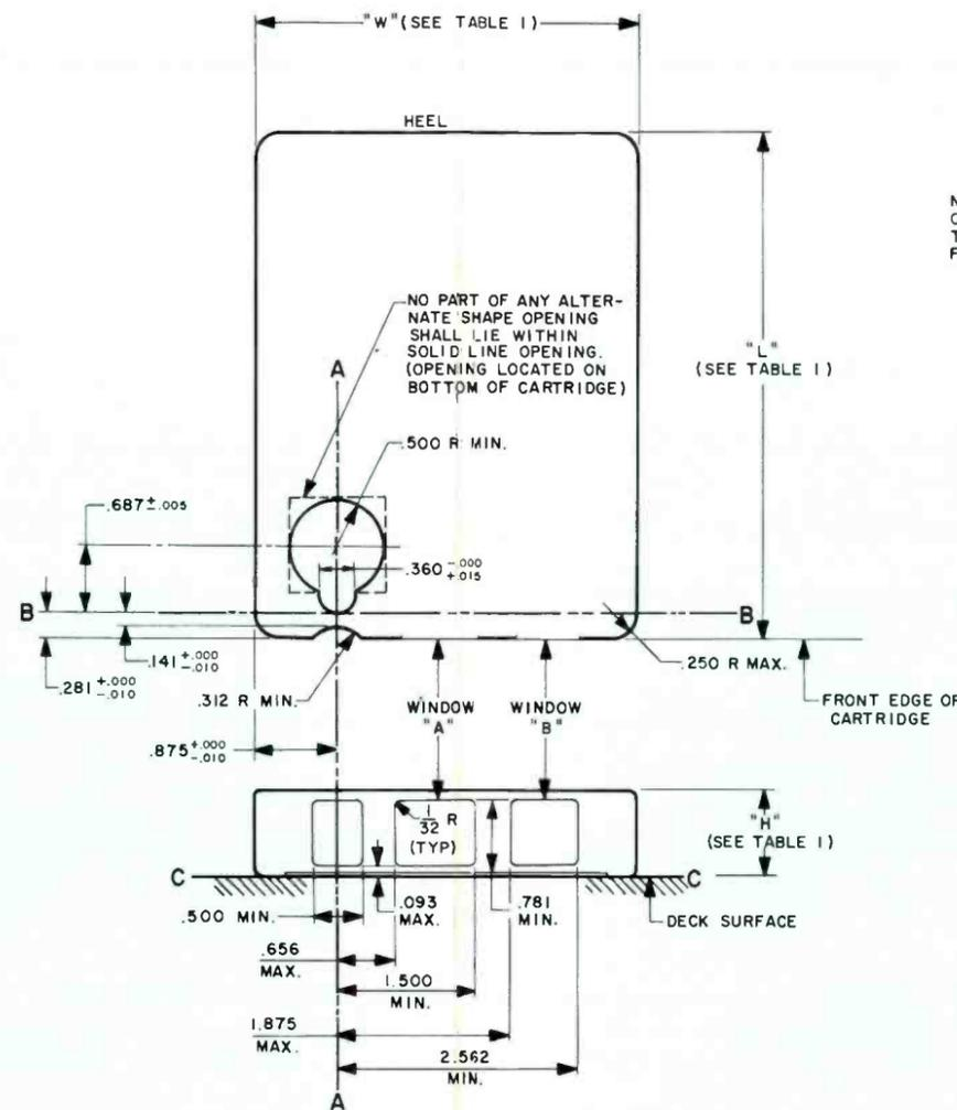
FIG. 3 CARTRIDGE DIMENSIONS
