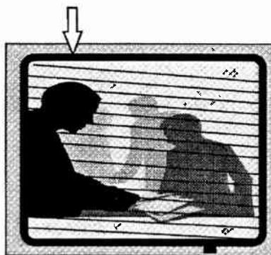
Video Signals are transmitted at 30 frames per second with 2 vertical scans per frame = 60 vertical scans per second.
