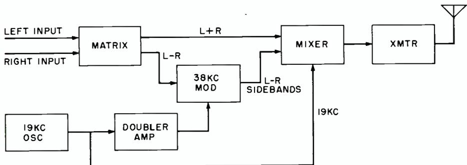
FIG. 5. Block diagram of stereo multiplex transmitter.
