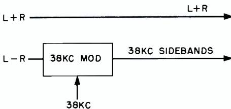
FIG. 4. Diagram showing  $L - R$  signal path.
