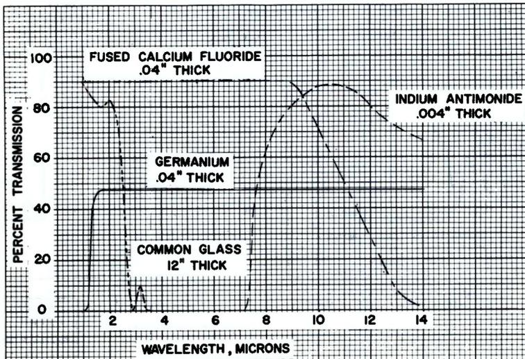
FIG. 6. Infrared transmission curves for various materials.
