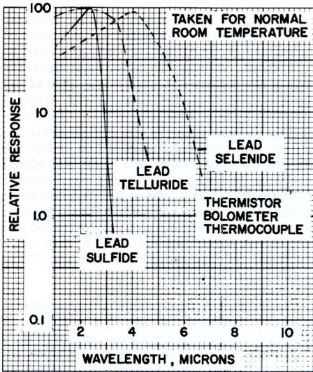
FIG. 2. Spectral responses of various infrared detectors.
