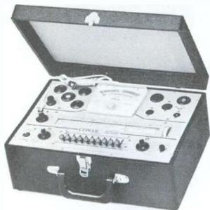
Model 220 tests old and new tube types including Nuvistors, Compactrons, 10-pin miniatures. Triple window, hi-speed illuminated roll chart lists over 1,000 tube types. Satin finish aluminum panel with etched black lettering. Durable black leather-fabric case; removable hinged lid. Top quality U. S. made components throughout. Easy to build and use. Size: 10-1/2" x 15-1/4" x 4-3/4". Shipping weight: 12 lbs. parcel post. 110-125 volts AC only. Kit Price - \$46.25. Assembled Price - \$57.00.
