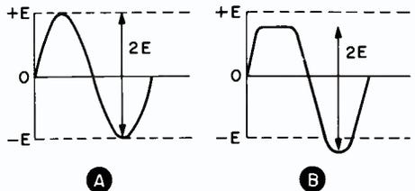
FIG. 1. Sine wave, A; sine wave with second harmonic distortion, B.
