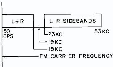
FIG. 6. Frequency distribution of FM multiplex signal.
