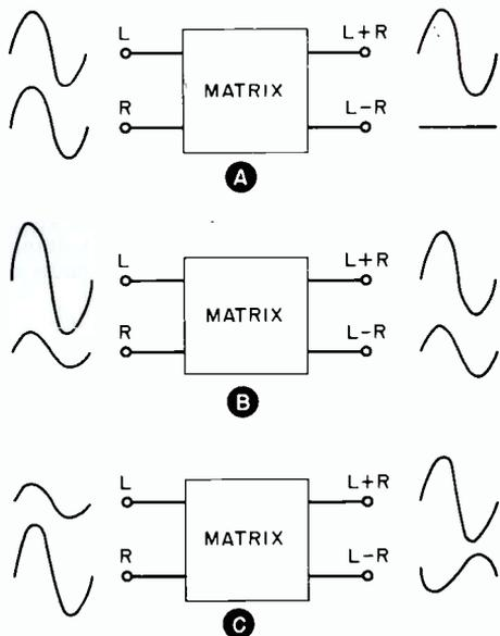
FIG. 3. Matrix input and output signals when (A)  $L$  is equal to  $R$ , (B)  $L$  is greater than  $R$  and (C) when  $R$  is greater than  $L$ .
