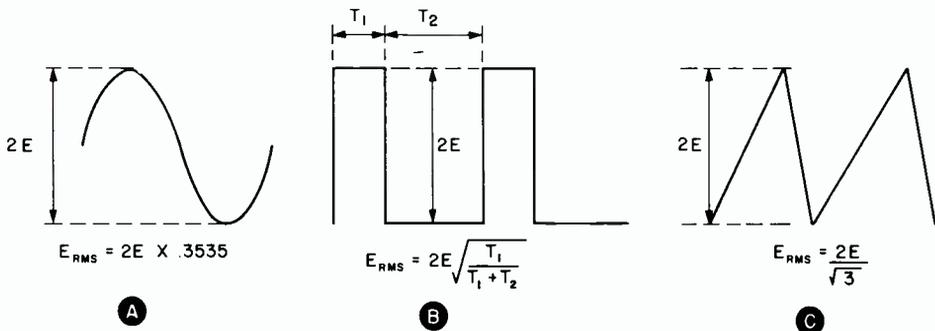
FIG. 3. Relationship between peak-to-peak and RMS for sine wave, A; rectangular wave, B; sawtooth, C.
