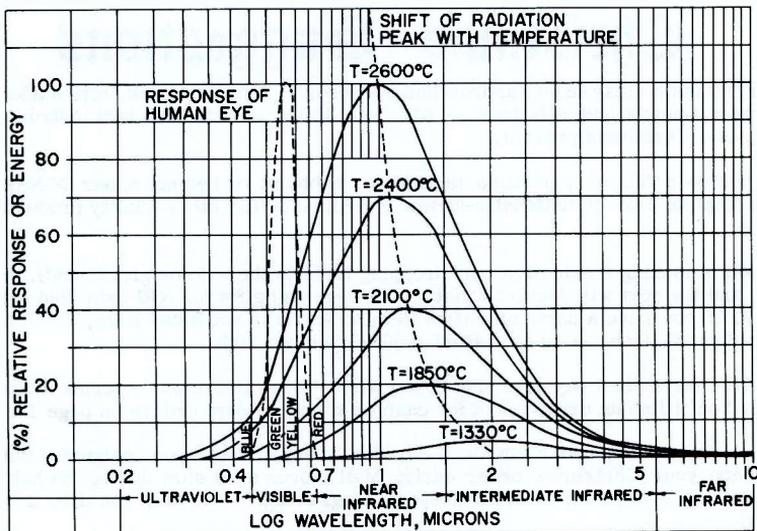
FIG. 1. The Visible and Infrared Spectrum.
