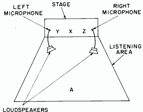
FIG. 1. Basic stereo system.
