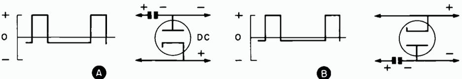
FIG. 4. Peak reading circuit connected to measure negative peaks, A; positive peaks, B.
