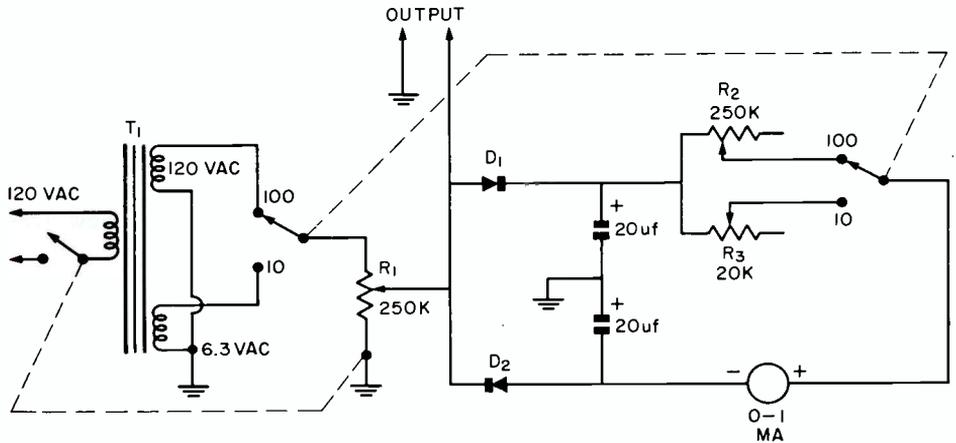
FIG. 8. Scope calibrator diagram.
