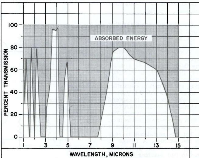
FIG. 5. Normal atmospheric infrared transmission over a one-mile path.
