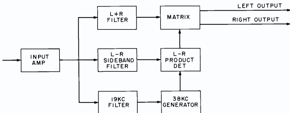
FIG. 7. Block diagram of FM multiplex adapter.
