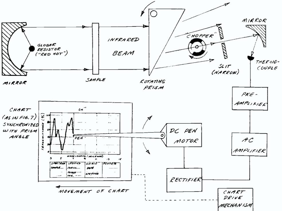
FIG. 8. Simplified infrared spectrophotometer.
