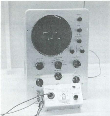
FIG. 10. Calibrator connected to produce 100V PP signal.
