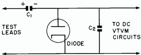
FIG. 2. AC portion of a typical vtvm.
