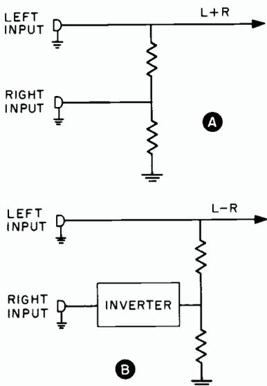
FIG. 2. Simplified matrix circuit.
