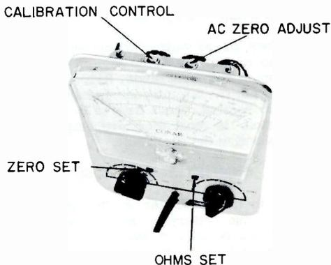
Model 211 VTVM showing the calibration controls.
