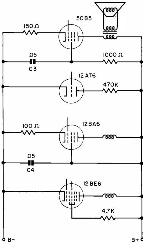
FIG. 6. Parallel branches of an AC-DC receiver.
