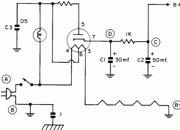
FIG. 5. AC-DC power supply.
