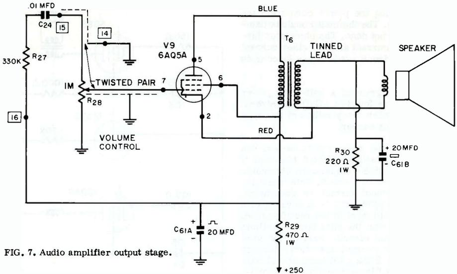
FIG. 7. Audio amplifier output stage.
