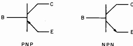
FIG. 1. PNP and NPN transistor symbols.
