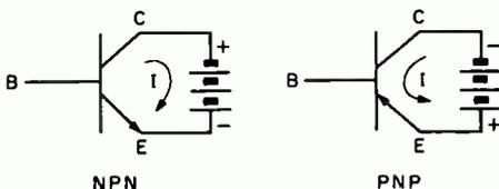
FIG. 2. Collector-emitter voltages.
