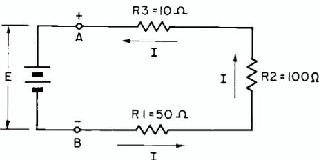
FIG. 2. Series circuit.
