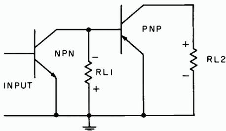
FIG. 8. Direct coupled NPN/PNP amplifier.
