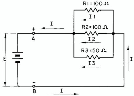
FIG. 3. Parallel circuit.
