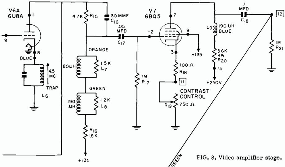
FIG. 8. Video amplifier stage.
