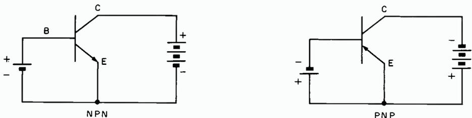
FIG. 3. Properly biased transistors.
