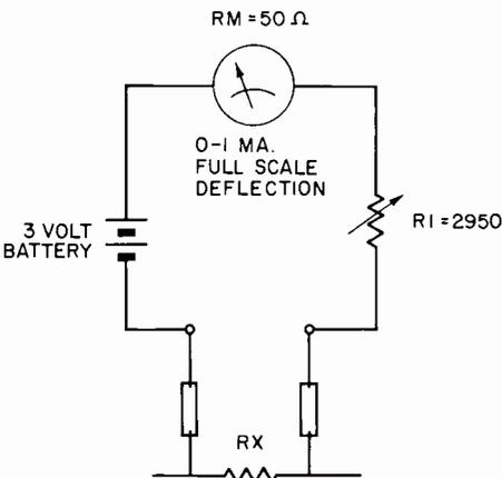
FIG. 1. Basic ohmmeter circuit.
