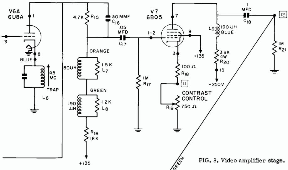
FIG. 8. Video amplifier stage.
