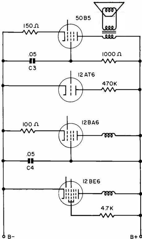
FIG. 6. Parallel branches of an AC-DC receiver.
