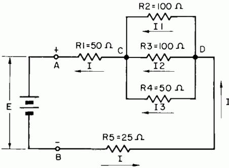
FIG. 4. Series-parallel circuit.
