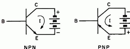
FIG. 2. Collector-emitter voltages.
