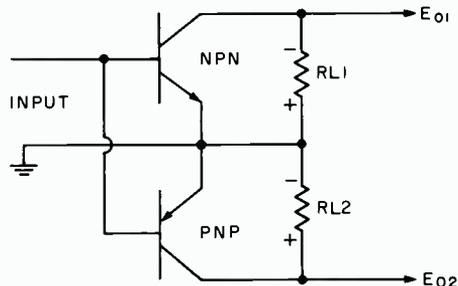
FIG. 7. Complementary symmetry phase inverter.
