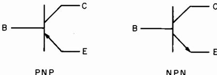
FIG. 1. PNP and NPN transistor symbols.
