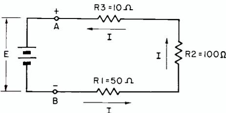
FIG. 2. Series circuit.
