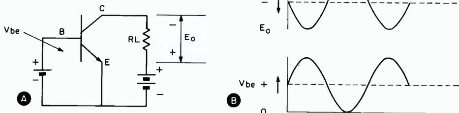
FIG. 4. Phase relations in a CE stage.
