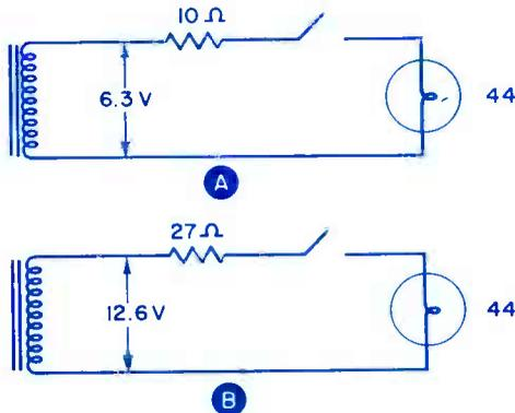
FIG. 1. Circuits for reducing turn-on surges by use of series resistor.
