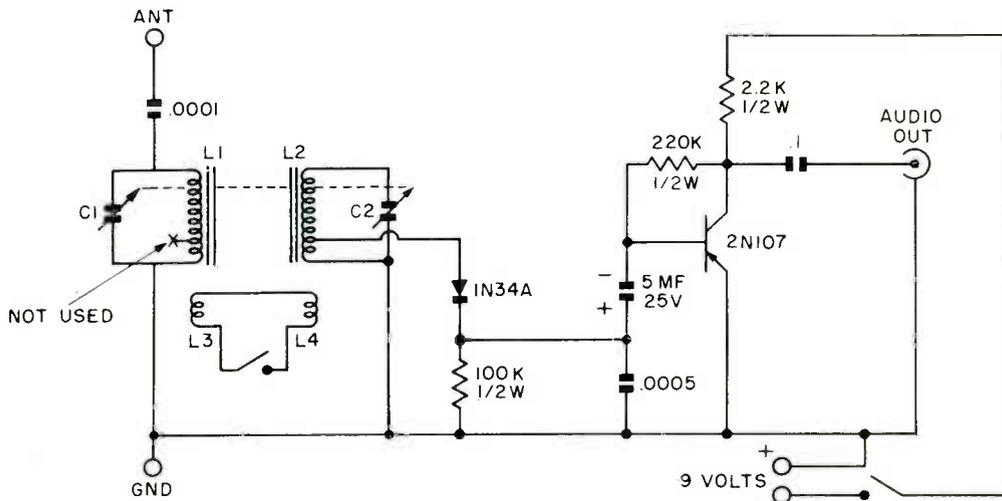
FIG. 5. The circuit of an AM tuner capable of providing top quality reception. C1 and C2 are 365 mmf variable (ganged). L1 and L2 are loopsticks (Allied Radio No. 91-C-057 or equiv.).
