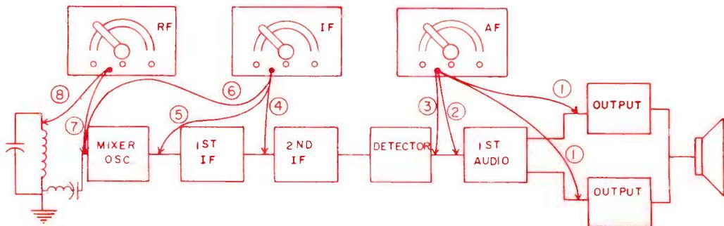
FIG. 5. How to use a signal generator to find a weak stage in a transistor set. The output of the signal generator is set to the correct frequency and moved from stage to stage to check loss in gain.
