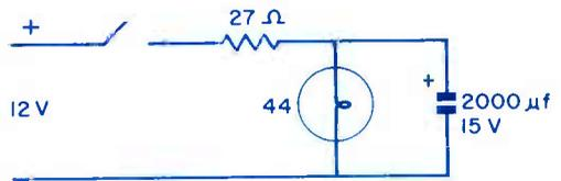
FIG. 2. Elimination of turn-on surge by use of R-C circuit.
