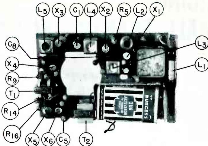
FIG. 1. Top view of the chassis of a transistor portable receiver showing the parts layout.
