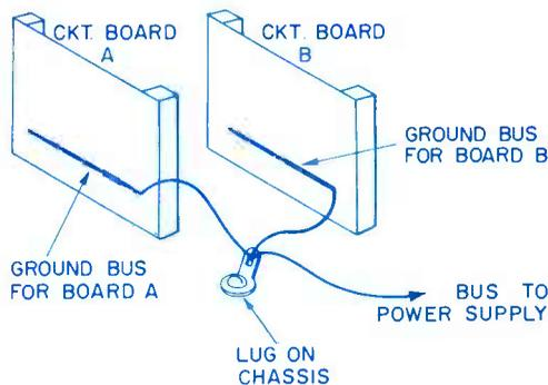
FIG. 5. Two circuit boards showing common bus for each board. Note that boards and power source are referenced to a central point to eliminate circulating chassis currents.
