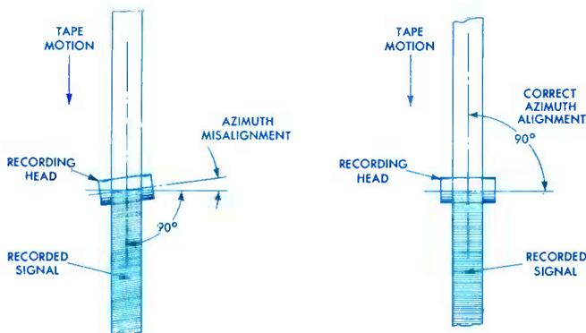
Recording and playback heads must be exactly perpendicular to motion of tape (as shown in the right hand sketch), for minimum distortion and maximum frequency response.
