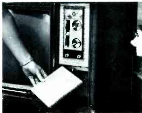
The bottom half of the right hand panel is removable to reveal the color convergence controls.
