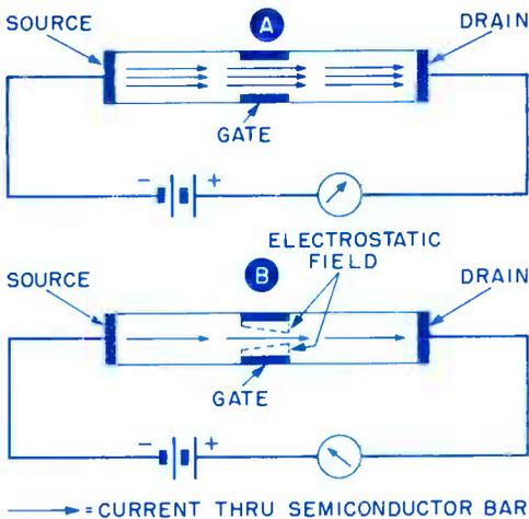
FIG. 2. The current flow through the bar from source to drain is due to the field effect.
