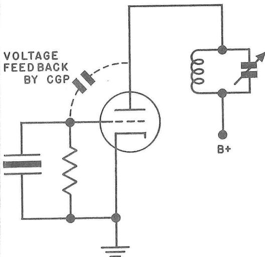
Examining the circuit, we see that it is essentially a tuned plate-tuned grid oscillator. The grid tank circuit is a mechanical tank, our crystal.
