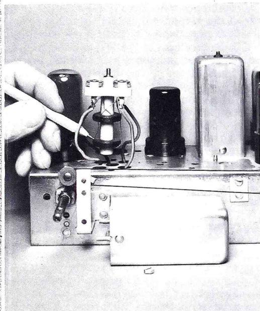
The pencil points to one of the coils in the i-f transformer. Carefully push the bottom coil a little closer to the top one to increase the bandpass of the receiver.
