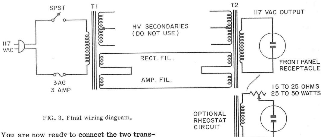
FIG. 3. Final wiring diagram.
