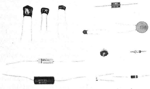
FIG. 1. Capacitor types.
