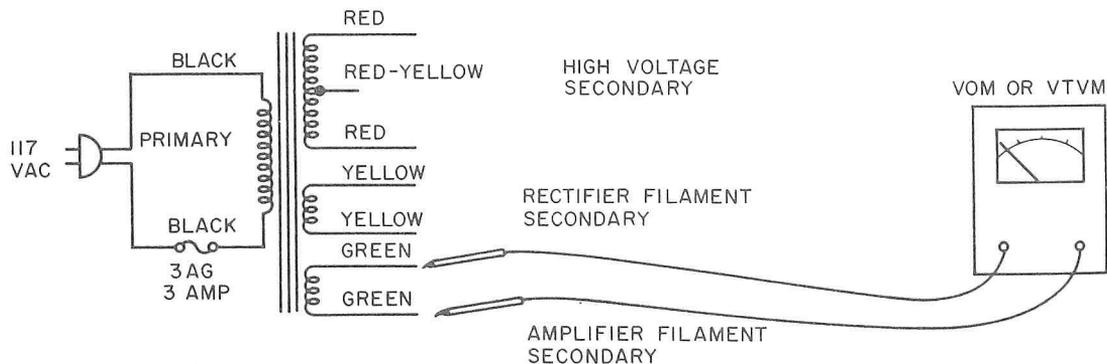
FIG. 1. Measure secondary voltages.
