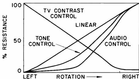
FIG. 2. Potentiometer tapers.
