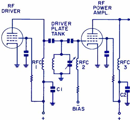
FIG. 5. Use of rf chokes in transmitter.
