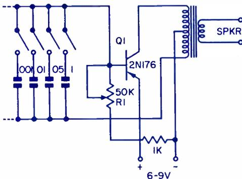
FIG. 5. A simple audio oscillator.
