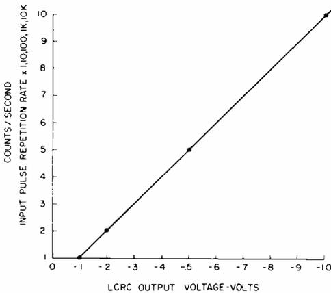
Fig. 2. Graph of input pulse rate vrs. output voltage.
