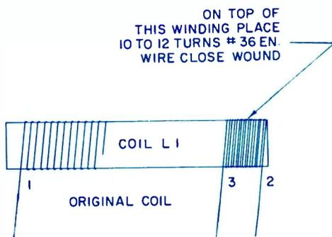
FIG. 3. Extra turns are placed in the position shown for feedback.
