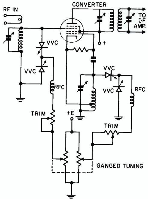
FIG. 3. Fine tuning accomplished by varying DC supply voltage.
