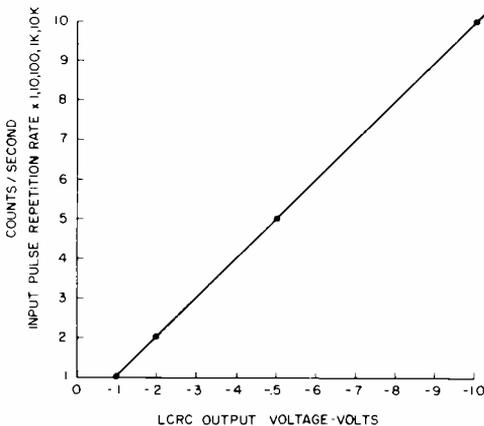
Fig. 2. Graph of input pulse rate vrs. output voltage.
