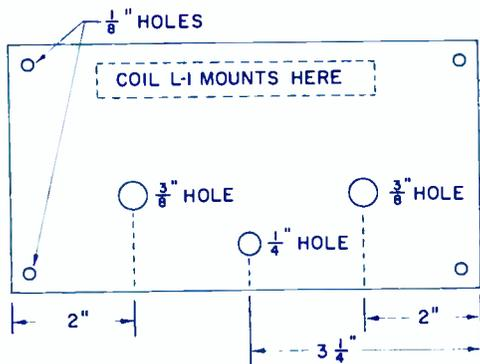
FIG. 2. Drilling of holes in perforated board.
