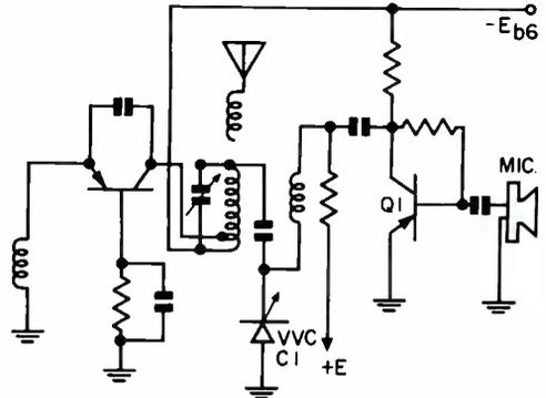
FIG. 4. The VVC used in a frequency modulation setup.
