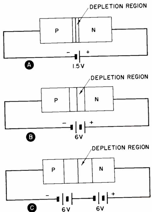
FIG. 1. The depletion region acts as a dielectric of a capacitor, A; widening the depletion region reduces the capacity, B; capacity further reduced by increased reverse bias, C.
