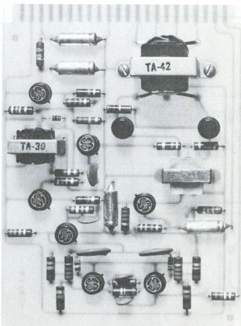
FIG. 5. Printed circuit board of Howler.
