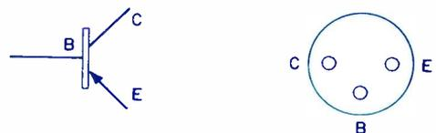
FIG. 6. Transistor connections.
