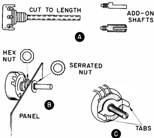
FIG. 3. Potentiometer mounting: (A) Hollow extension shaft; (B) double-nut mounting; (C) twist-tab mounting.
