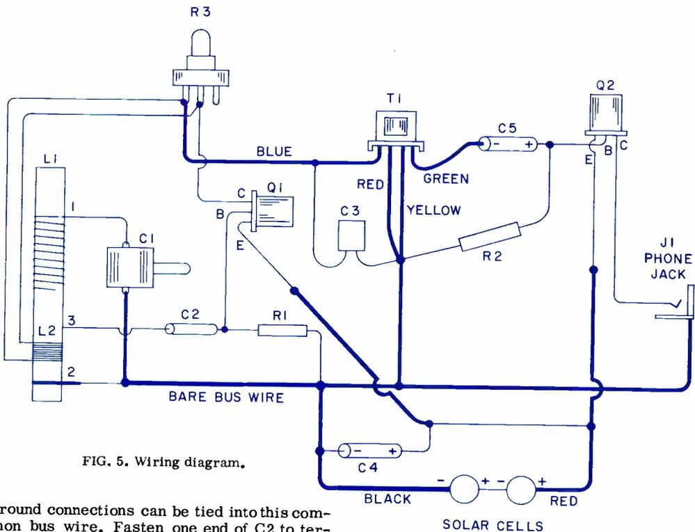
FIG. 5. Wiring diagram.
