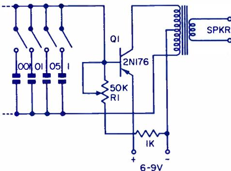
FIG. 5. A simple audio oscillator.
