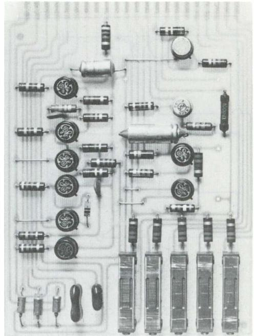
FIG. 3. Printed circuit board of LCRC.
