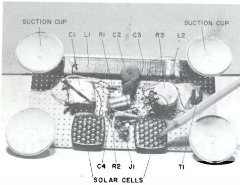
FIG. 4. Wiring of receiver with solar cells shown in lower center. The four suction cups to hold the radio against the window pane are seen at the corners.
