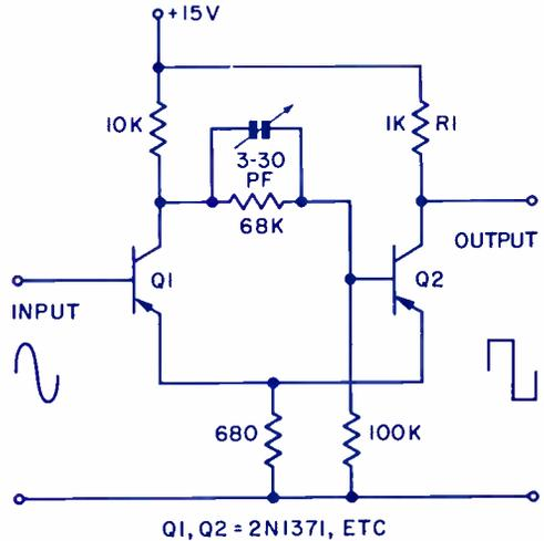
FIG. 6. Transistorized clipper producing square waves from sine wave input.
