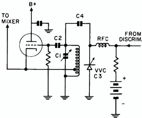
FIG. 2. Oscillator frequency controlled by DC voltage from the discriminator.
