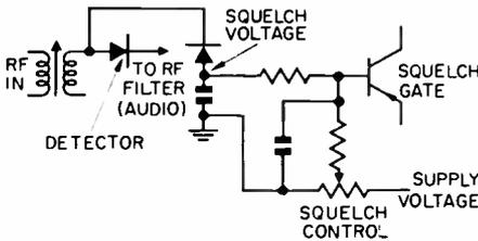
gate tube or transistor. When no carrier is present, the audio stage is cut off and none of the noise is allowed to pass. When a carrier pops on the air, the diode rectifies it, producing bias which overcomes the cutoff bias. The gate is open and sound emits.
