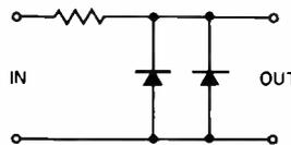
adding another diode and the level may be controlled by inserting bias voltages (as in the limiter) to set the clipping level.
