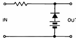
a predetermined point as set by the bias battery. This same arrangement may be used to square a sinusoidal waveshape by simply
