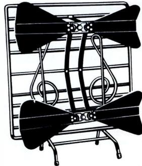
FIG. 2. Periodic type indoor antenna is highly directive, delivers 10 db gain over isotropic.
