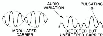
retained half is pulsations whose amplitudes are varying at an audio rate. The higher frequency component is filtered by a network and the result is a current which varies at an audio rate.
