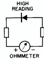
is the quickest method—simply measure the diode in one direction, then reverse the leads. The resistance should be at least 10 times greater in one direction than it is in the other. If the polarity of the ohmmeter leads is known, the cathode and anode may be determined. With the positive lead on the anode and the negative on the cathode, the lowest resistance reading will be obtained.
