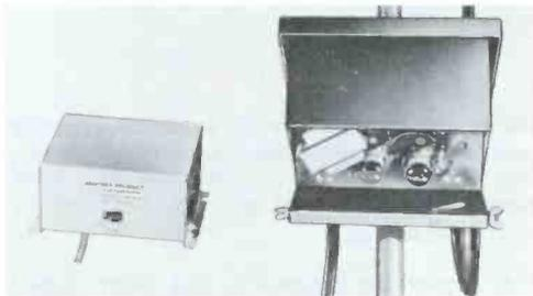
FIG. 9. UHF amplifiers of this type are expensive, yet cover only a portion of UHF band.
