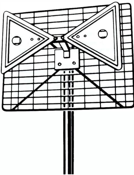
FIG. 3. Bowtie-with-screen type outdoor UHF antenna.
