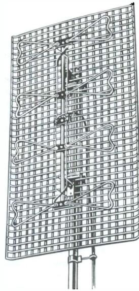
FIG. 4. Bowtie-with-reflector type outdoor UHF antenna.
