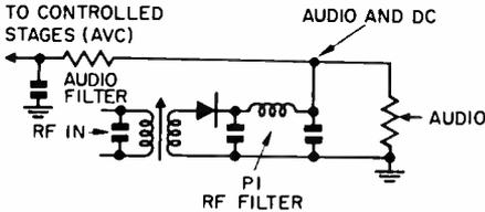
tor diode in most cases), and causes a changing DC to be applied to the previous rf and i-f amplifiers in accordance with the carrier amplitude variation. This tends to hold the level constant. If the carrier level increases, the bias increases, decreasing the gain of the stages it is applied to, and vice versa.
