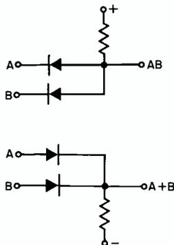
and operate like this. In the case of the AND gate, if an input appears at A and B, an output will be present. If A appears but B does not, no output. The OR gate gives an output for either A or B.
