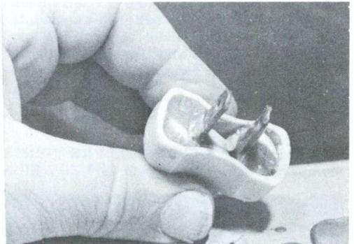
You can make an extension cord plug shock-and-short proof by the simple expedient of melting wax from an ordinary candle around it. Here it is seen that the bared ends of the wire are imbedded in melted wax which has hardened. A film of wax on the prongs of the plug will make it slip in and out of the receptacle easier.
