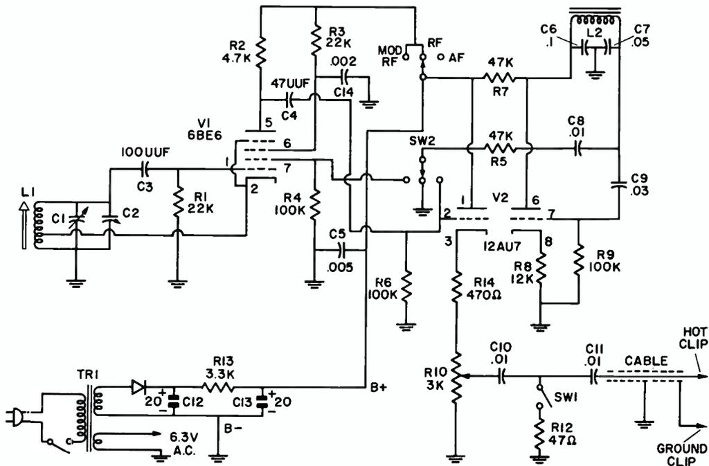
FIG. 2. Simplified diagram of the CONAR Model 280 circuit.
