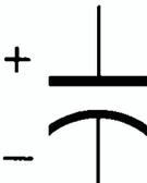
and will always have one side designated as the positive and one as the negative lead. It is polarized and this dictates the applications in which it may be used. The dielectric is the product of an electro-chemical process and forms between the plates of the capacitor when a voltage is applied. This voltage is known as the forming voltage.
