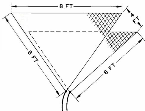
FIG. 2. Conventional horn rotated 90 degrees.
