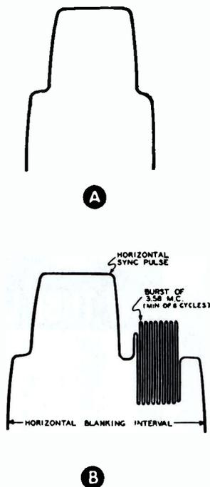
FIG. 1. A is the sync pulse transmitted for a black and white picture; B the sync pulse for color.
