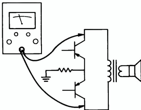
FIG. 6. The VTVM set for AC measurements may be connected to the collector leads of output transistors, or you can get by with a smaller signal from either collector lead to chassis.
