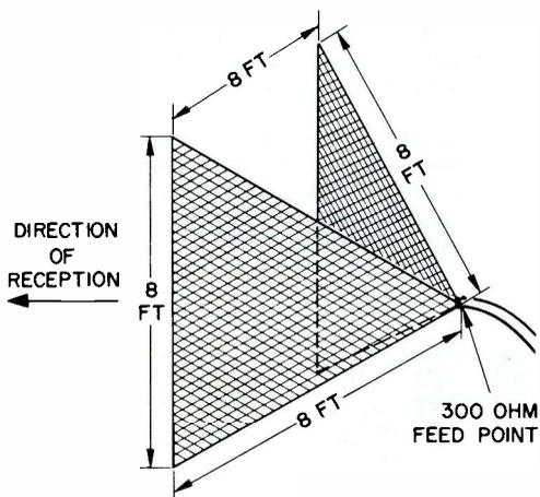
FIG. 1. Conventional design having "chicken wire" netting as the conductor.
