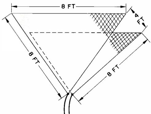
FIG. 2. Conventional horn rotated 90 degrees.
