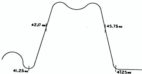
FIG. 3. Response curve of a typical video i-f in a color receiver.
