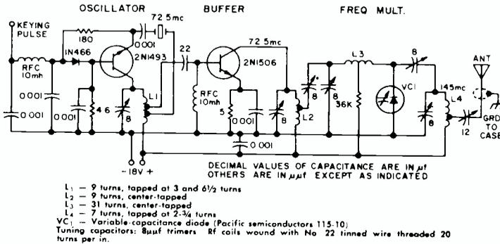
The OSCAR transmitter circuit.
