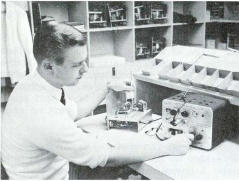
FIG. 8. Technician Jim Johnson of NRI's Quality Control calibrates an assembled 280 Signal Generator by beating its signals against a special crystal-controlled standard.
