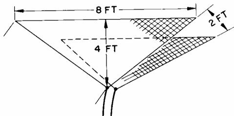
FIG. 3. Design for a "short-horn" antenna.
