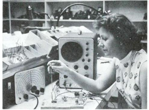
FIG. 9. Helen Gillespie of Assembly pre-adjusts the trimmers to be used in a CONAR 280 Signal Generator kit. Proper adjustment produces a circular pattern on the scope screen.
