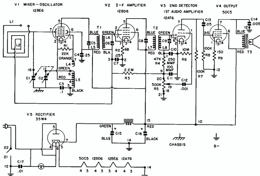
FIG. 7. Schematic diagram of a typical AC-DC radio receiver.
