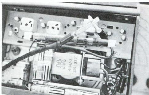
FIG. 10. Closeup showing how hot and ground leads of the 280 are clipped together and slipped over a loopstick in a transistor set.
