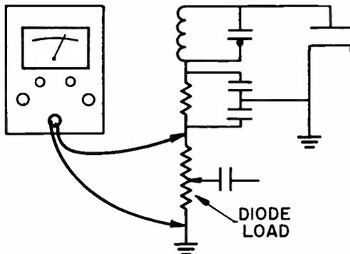
FIG. 4. Here the DC VTVM is connected across the volume control to observe the effect of the RF signal level at the detector output.
