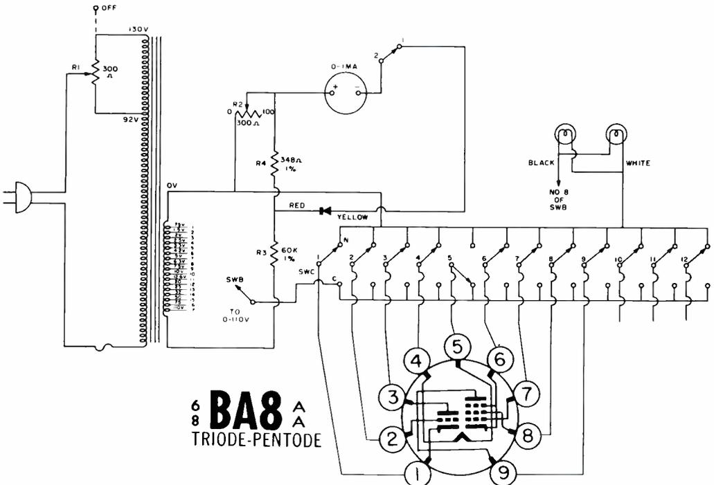
Fig. 4. Setup for line voltage adjustments and filament voltage.
