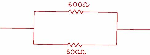
Fig. 8. Find value of two resistors in parallel.
