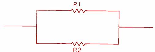
Fig. 9. Find the parallel resistances of  $R_1$  and  $R_2$  if  $R_1$  equals 6 ohms and  $R_2$  equals 8 ohms.
