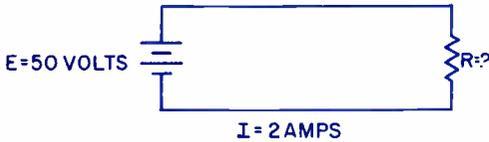
Fig. 3. Find R in this simple series circuit.
