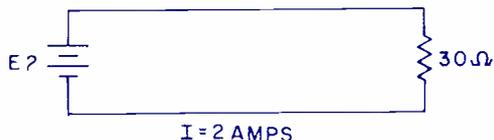
Fig. 1. A simple series circuit.
