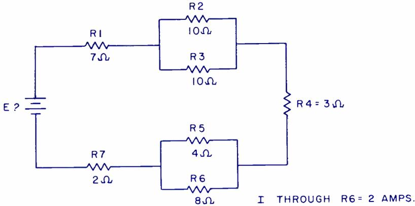
Fig. 10. Find the applied voltage  $E$  in the circuit shown.
