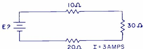
Fig. 2. Find the voltage when three resistors are in series.
