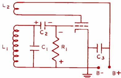
In this circuit, when the power is applied plate current will begin to flow. The current flowing through L2 will produce a changing magnetic field which will induce a voltage into L1. The induced voltage charges C1, which starts the oscillation in the tank circuit (L1-C1). The voltage across C1 becomes the grid voltage because the value of C2 is so large that its reactance is small at the frequency of oscillation. In effect, C1 is connected directly to the grid.
