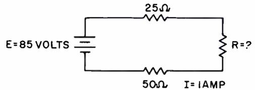
Fig. 4. Find the value in the unknown resistor.
