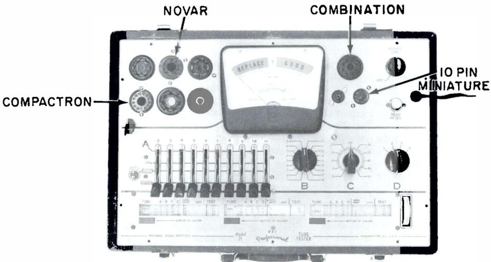
Photo of a modernized old tube tester.
