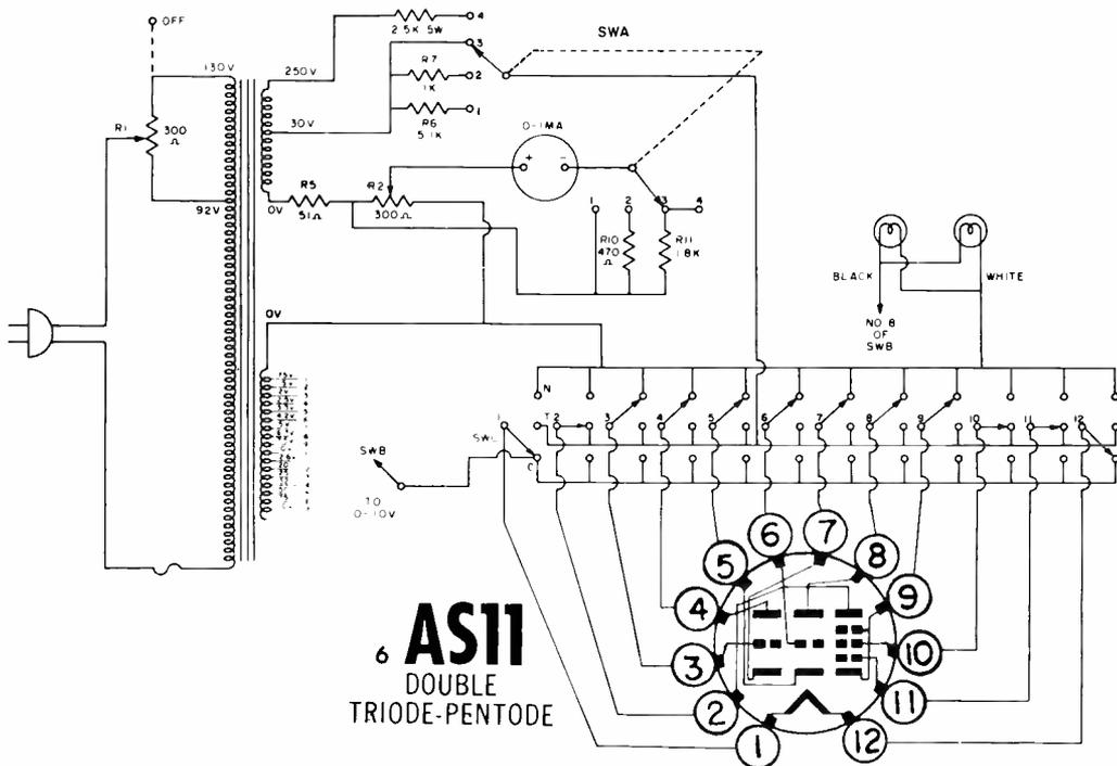
Fig. 6. Testing the pentode section of a compactron for emission.
