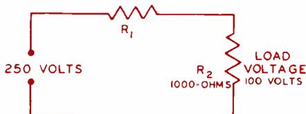
The first method you could use to determine the size of the series resistance is to use Ohm's Law to find the current in the circuit and then to find the value of the resistance. You know that the load will drop 100 volts and the resistance is 1,000 ohms. Dividing 1,000 ohms into 100 volts ( $I = \frac{E}{R}$ ) gives you .1 ampere.
