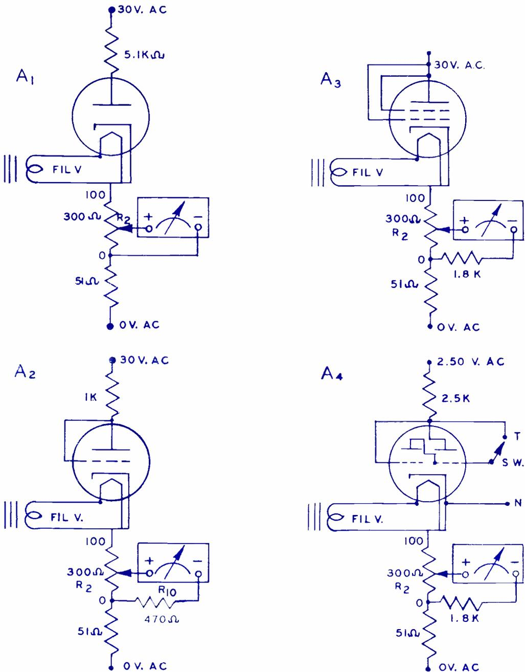
Fig. 7. Basic setups to check cathode emission.
