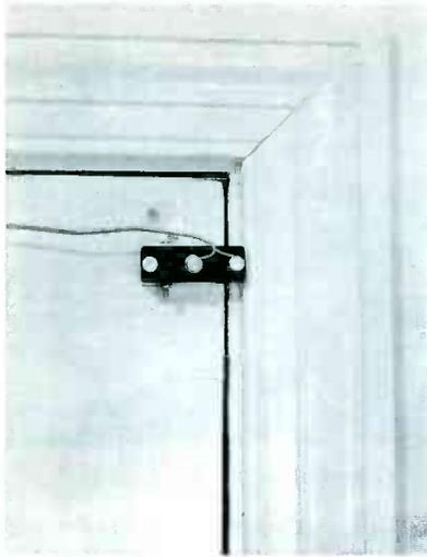
Fig. 7. Microswitch installed on door.
