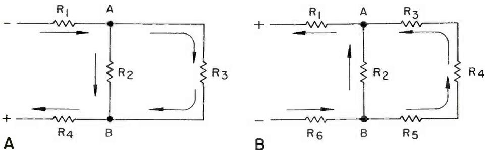
Fig. 3. Identifying various circuits by assigning polarity designations and tracing the path of current flow.
