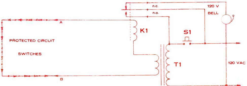
Fig. 1. Basic circuit (See parts lists with Fig. 8.)
