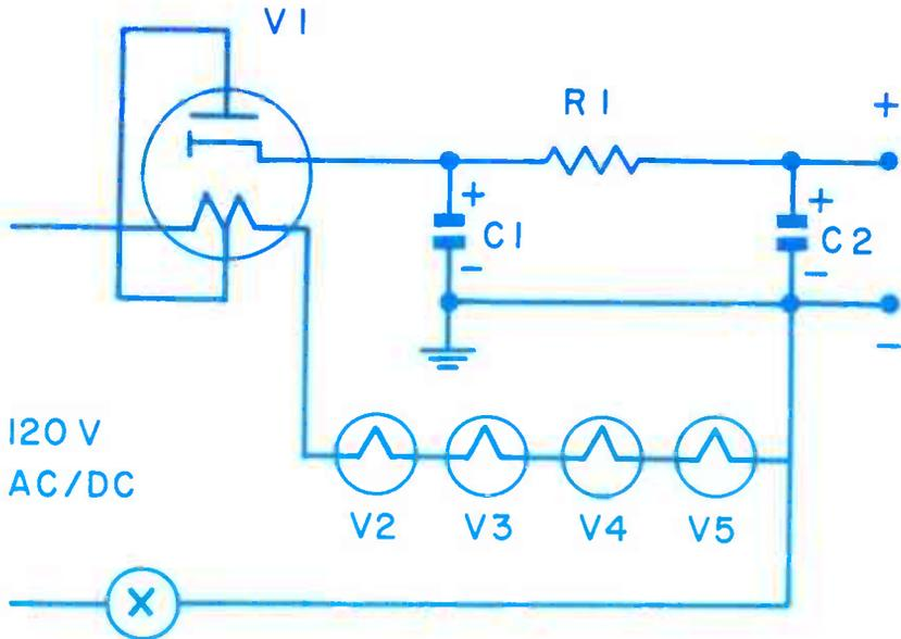
Fig. 5. A typical ac-dc power supply.
