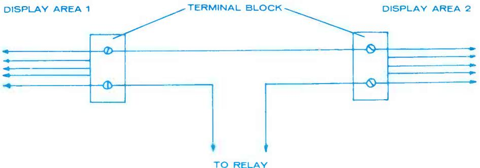
Fig. 4. Connecting two or more terminal blocks.
