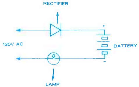
Fig. 11. Simple battery charger.
