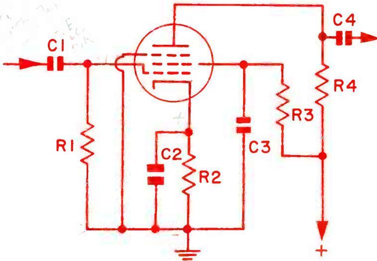
Fig. 1. A typical pentode stage.
