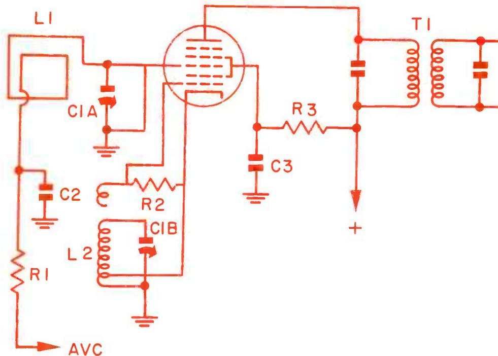
Fig. 4. A typical mixer-oscillator stage.
