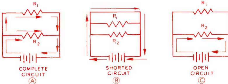
Fig. 1. Differences between an open circuit and a short circuit.
