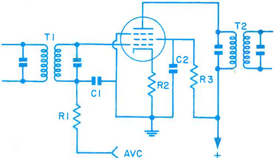
Fig. 3. A typical i-f stage.
