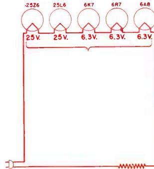
Fig. 2. A series circuit with current flowing through all points.
