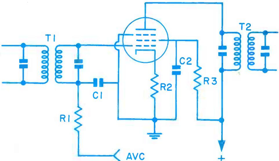
Fig. 3. A typical i-f stage.
