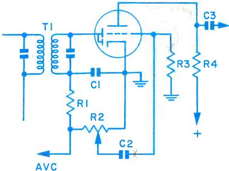
Fig. 2. A typical second detector-first audio stage.
