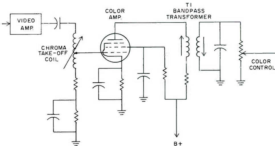
Figure 7. Bandpass amplifier circuits of a typical color receiver.
