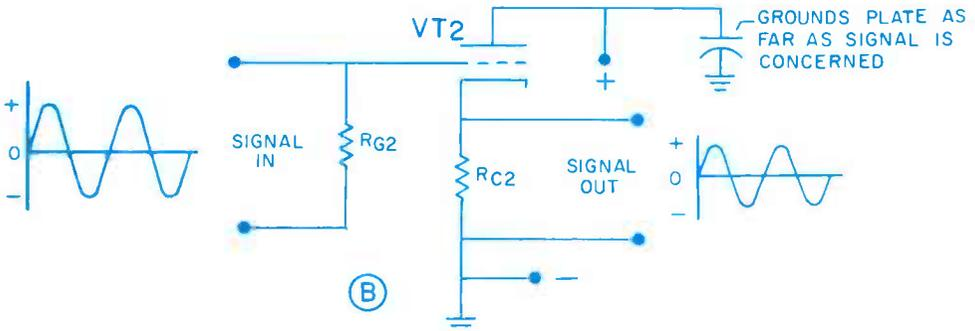
Figure 10B. Grounded plate circuit gives gain less than 1 but with no phase reversal.
