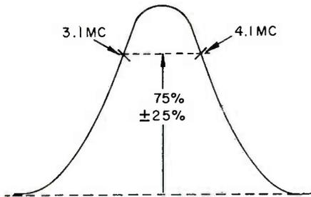
Figure 6. VSM response curve for a typical color receiver.
