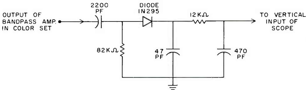
Figure 5. Detector circuit for demodulating the swept signal.
