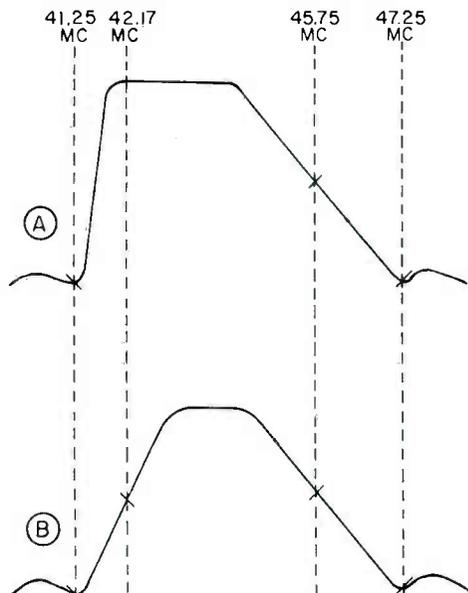
Figure 1. Video i-f response curve for a broadband receiver (A) and for a narrow-band receiver (B).
