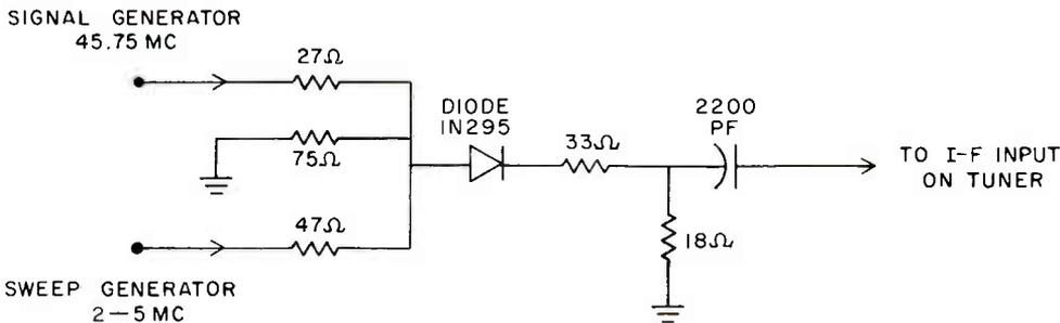
Figure 4. Schematic diagram of Modulator.
