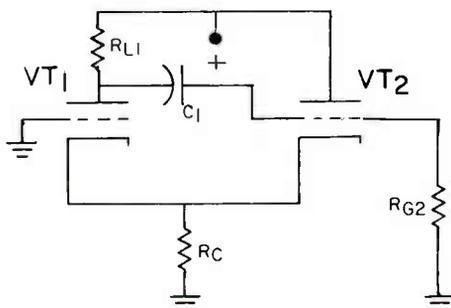
Figure 12. Basic cathode coupled multivibrator. The frequency of operation is determined by  $C_1$  and  $R_{G2}$ ,  $R_{L1}$  being so small compared to  $R_{G2}$  as to have little or no effect on the frequency.
