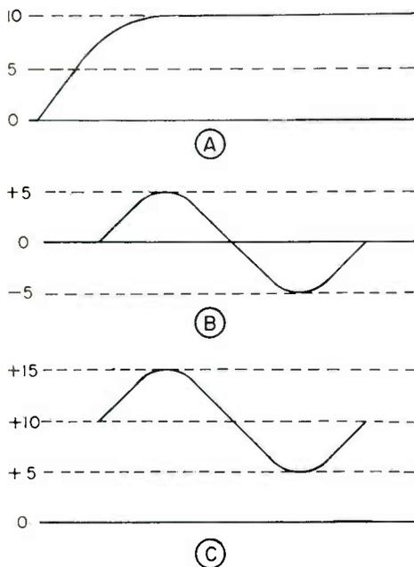
Fig. A illustrates a typical dc voltage. Notice that it begins at zero and rises to a maximum constant value. Fig. B shows a typical ac voltage. It begins at zero and rises to a maximum positive value, returns to zero, reaches a maximum negative value, and returns to zero again.
