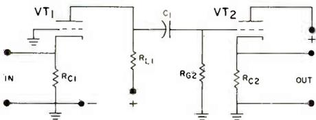
Figure 11. Although the gain of  $VT_2$  is less than 1, the output signal of  $VT_2$  is greater than the input signal of  $VT_1$  because of the gain in  $VT_1$ .
