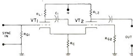
Figure 13. Typical cathode coupled multivibrator found in many electronic devices.
