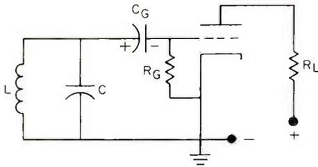
Figure 3C. The polarity of the dc voltage due to grid - cathode rectification is shown across capacitor  $C_G$ .
