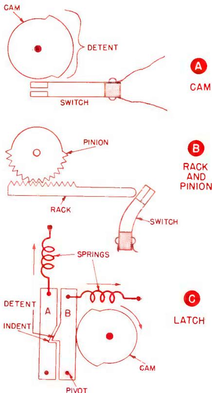
Fig. 5. (A) Cam; (B) Rack and Pinion; (C) Latch.
