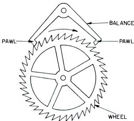
Fig. 4. A simple escapement mechanism.
