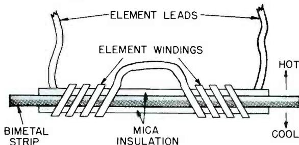
Fig. 3. Bimetal strip used to operate a mechanical timer.
