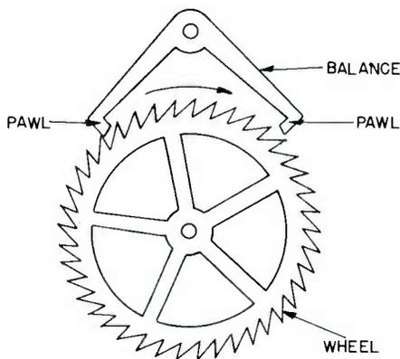
Fig. 4. A simple escapement mechanism.
