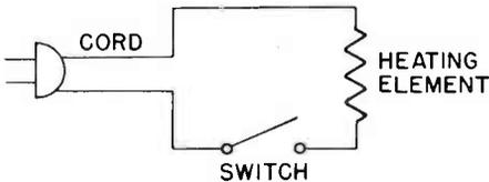
Fig. 1. The basic electrical circuit.
