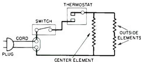
Fig. 2. Circuit position of thermostat.
