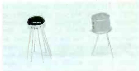
Fig. 5. Type 914 IC (left); TO5 transistor (right).
