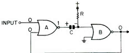
Fig. 10. Monostable multivibrator.
