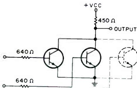
Fig. 2. RTL gate circuit.
