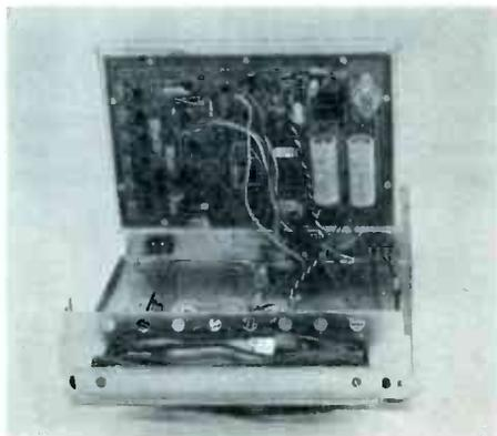
Fig. 18. Rear of CONAR Model 680 Color Generator with circuit board raised.
