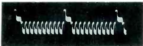
Fig. 16. Color bar video waveform at mixer output.
