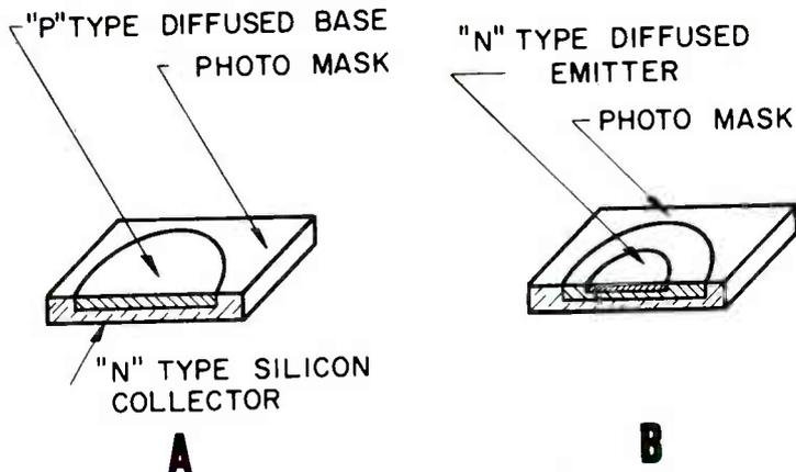
Fig. 1. Forming base (A) and emitter (B) in the planar process.
