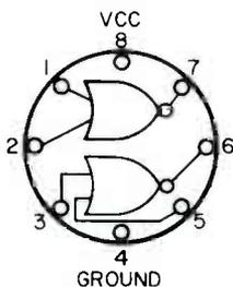
Fig. 4. Basing of 914 dual 2-input gate.
