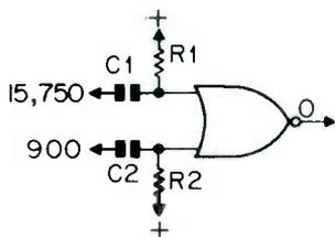
Fig. 13. Alternate line AND gate.
