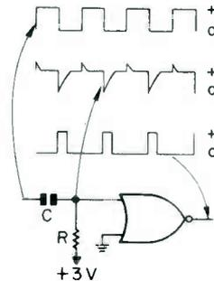
Fig. 9. Half a 914 connected as a shaper. while the second is connected through resistor R to the 3-volt line, making the output normally "zero". Applying a pulse input signal through capacitor C has the following effects:
