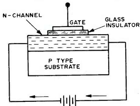
Fig. 5. Current flow through an insulated-gate, N-channel field-effect transistor with no bias applied.
