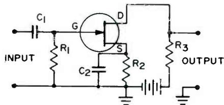
Fig. 3. An amplifier using an N-channel junction-gate FET.
