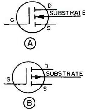
Fig. 8. The schematic symbols for the enhancement type of IGFET's. (A) An N-channel unit; (B) a P-channel unit.
