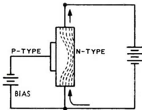
Fig. 1. Drawing showing the basic operation of a field-effect transistor.
