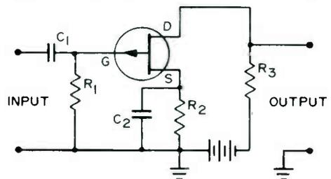
Fig. 4. An amplifier using a P-channel junction-gate FET.
