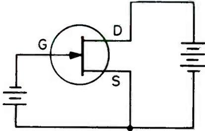
Fig. 2. Schematic representation of the circuit shown in Fig. 1.
