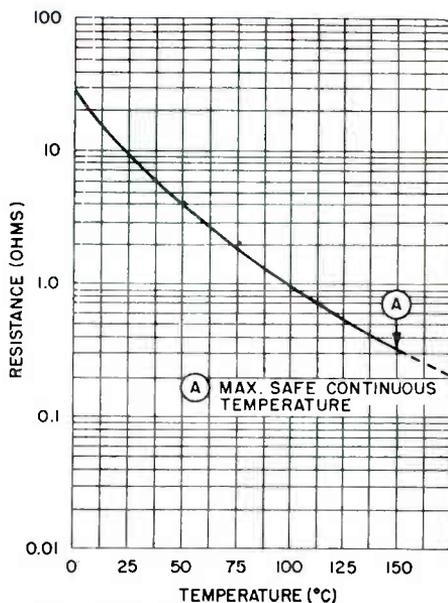
FIG. 2. Resistance-temperature curves of a typical thermistor.
