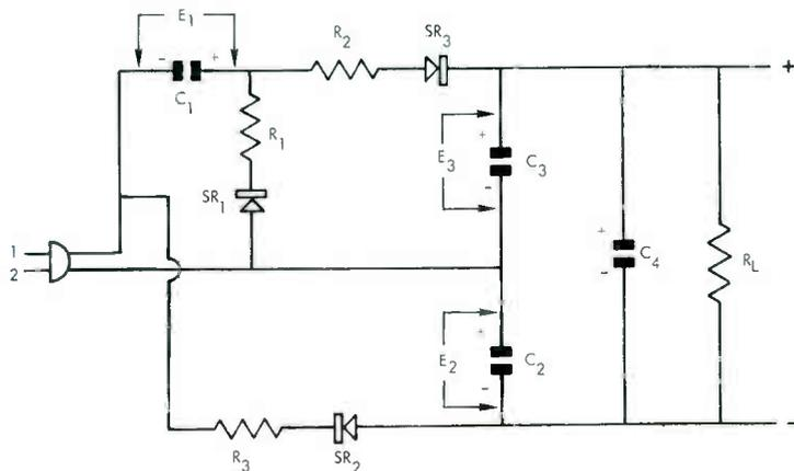
of  $C_3$  and away from the positive side through  $SR_3$ ,  $R_2$ ,  $C_1$  and the ac source in series. Thus  $E_3$  receives a charge equal to the peak value of the applied voltage plus  $E_1$ , making  $E_3$  equal to approximately twice the peak value of the applied voltage.
