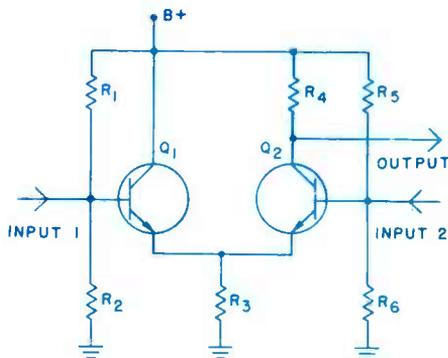
Fig. 1. Basic differential amplifier circuit.
