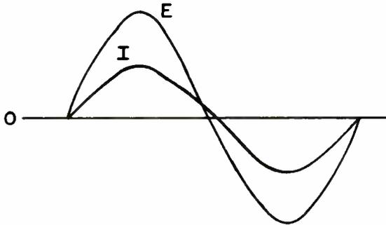
Fig. 1. Voltage and current waveforms are in phase in ac circuit containing only resistance.
