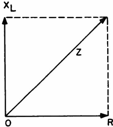
Fig. 4. Vector addition of a 10-ohm resistance and a 10-ohm inductive reactance.
