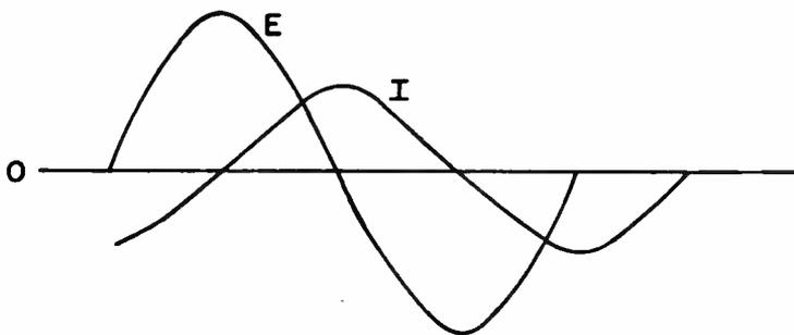
Fig. 2. Voltage and current waveforms in ac circuit containing only inductive reactance.
