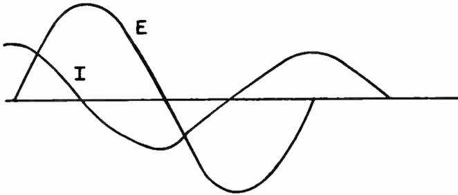
Fig. 3. Voltage and current waveforms in ac circuit containing only capacitive reactance.
