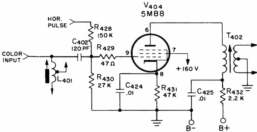
Fig. 8. Schematic diagram of a burst-gate amplifier stage.
