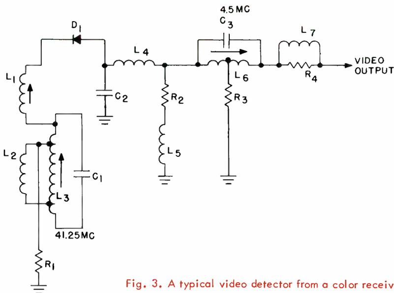
Fig. 3. A typical video detector from a color receiver.
