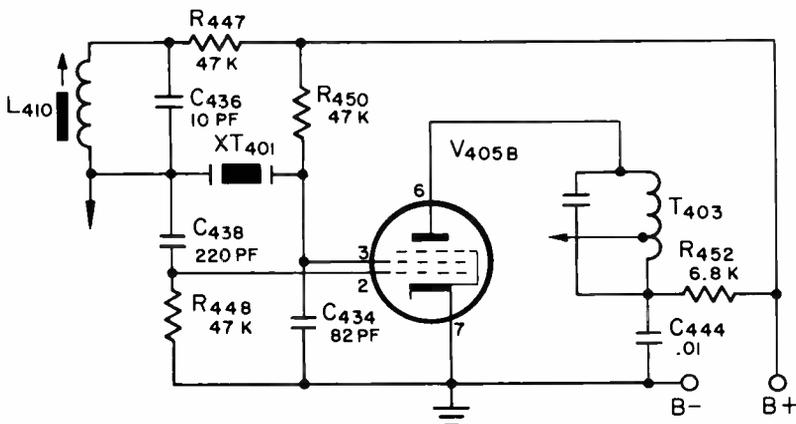
Fig. 7. Schematic diagram of a color oscillator.
