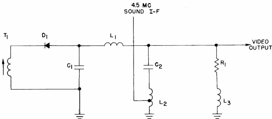
Fig. 2. A typical video detector from a monochrome receiver.
