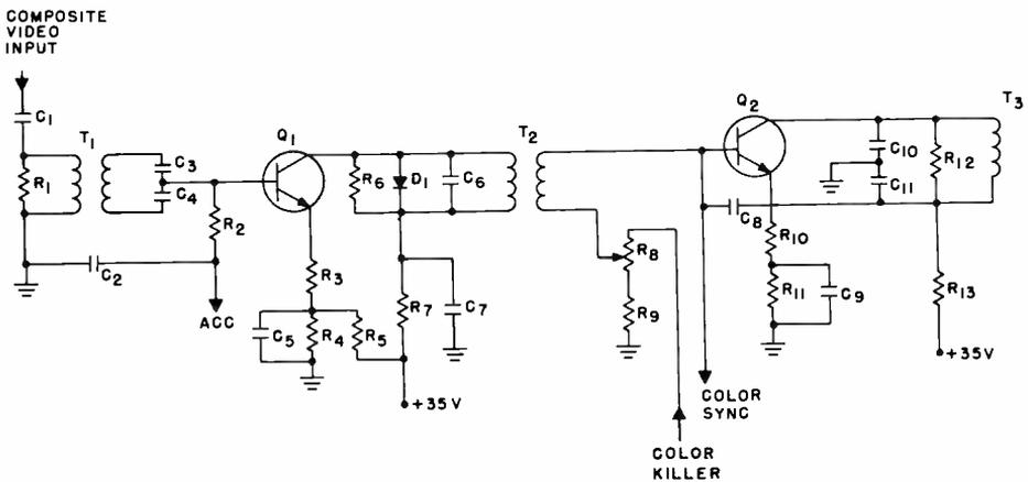
Fig. 9. A two-stage transistor color i-f amplifier.
