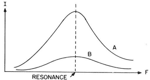
Fig. 7. A graph showing how the current in a series-resonant circuit is affected by resistance.
