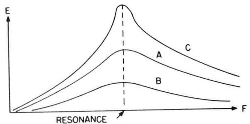
Fig. 8. A graph showing voltage versus frequency of series-resonant circuits with different L-C ratios.
