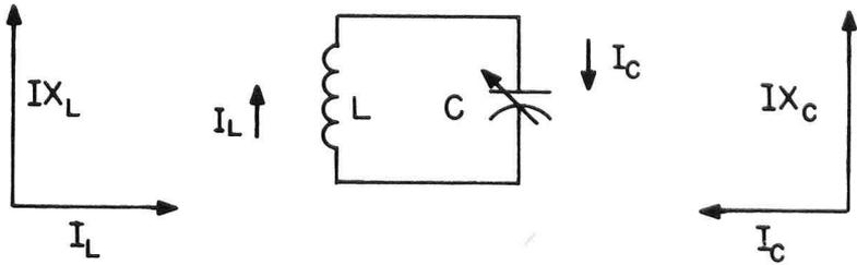
Fig. 6. Vector diagrams showing polarity of voltages across coil and capacitor.
