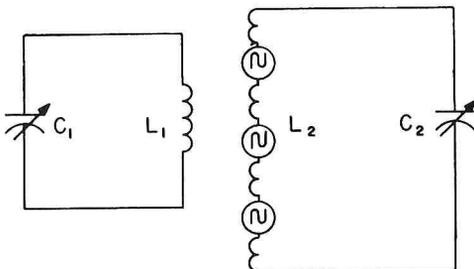
Fig. 5.  $L_2 - C_2$  is a series-resonant circuit.
