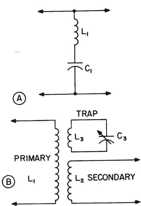
Fig. 9. Series-resonant circuits are often used as traps. The trap shown at B is called an absorption trap.
