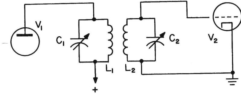
Fig. 4.  $L_2 - C_2$  form a series-resonant circuit producing a resonant voltage step-up.
