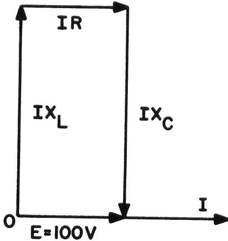
Fig. 3. Vector diagram of voltages in Fig. 1.
