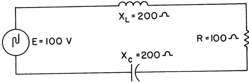
Fig. 2. A series-resonant circuit.
