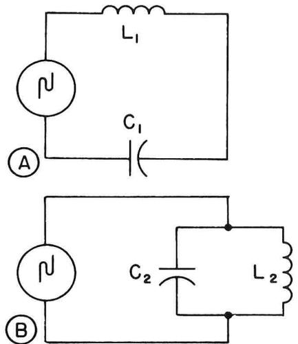
Fig. 1. A diagram of a series-resonant circuit is shown at A; a parallel resonant circuit at B.
