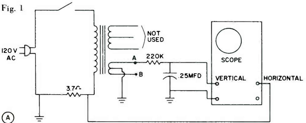
primary current can be disregarded. My first thought was to use a 5-ohm, .5-watt resistor, but my junk box came up with a 3.7-ohm, 5-watt resistor that worked just as well.
