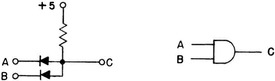
The inputs are bits that may be either binary one or zero. Just as we did with the OR gate, we can make a truth table for the AND gate that shows the output of all possible combinations of input conditions. Assume positive logic with levels of "1" = +5 volts and "0" = zero volts or ground. Using these levels and remembering that an AND gate produces a "1" output when all inputs are simultaneously "1", choose the correct truth table below.
