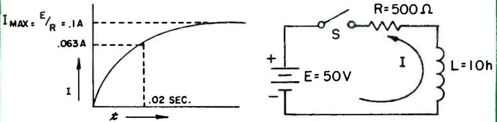
2. (.127 amperes) When the voltage is initially applied to the circuit, the rapidly expanding magnetic field in the coil generates an inverse EMF that opposes the applied voltage and keeps the current to zero. But as the field expands to its maximum, the induced voltage decreases and the current rises gradually. It takes a maximum of five time constants ( $5 L/R$ ) for the current to rise to its maximum value of  $E/R$ .
