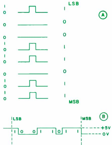
**Fig. 1. Parallel (A) and serial representation (B) of the binary word 11011001.**
