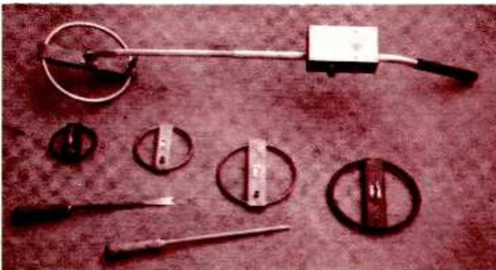
**Fig. 2. A beat-frequency metal locator with interchangeable coils and digging-tool accessories.**
