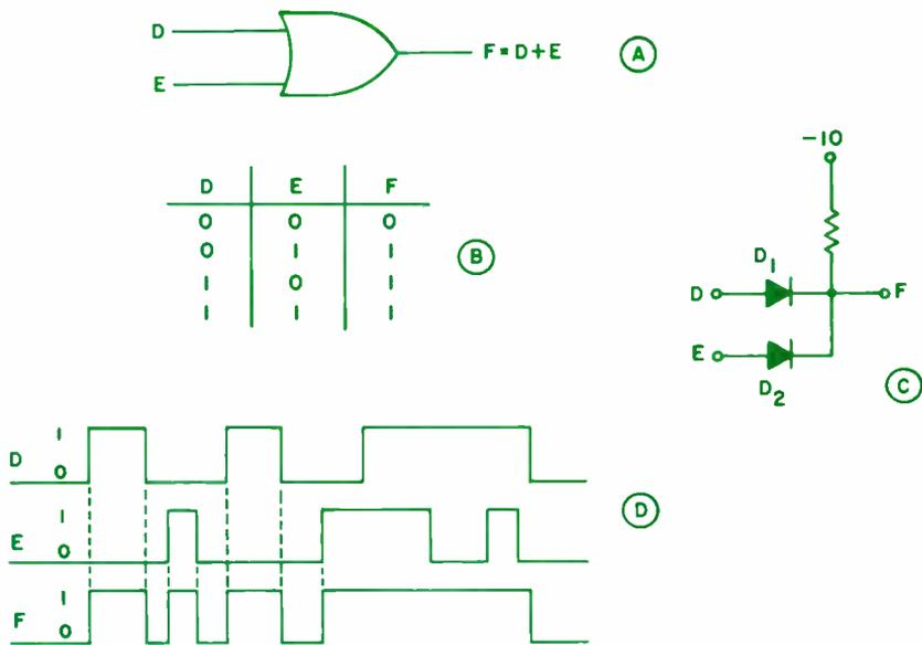
Fig. 4. OR gate symbol (A), truth table (B), circuit (C), and representative input/output waveforms (D).
