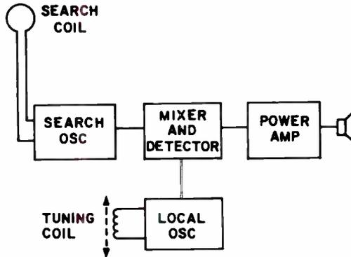
**Fig. 3. Block diagram of a typical beat-frequency metal detector.**
