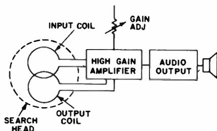
Fig. 5. Block diagram of an inductive-bridge metal detector.
