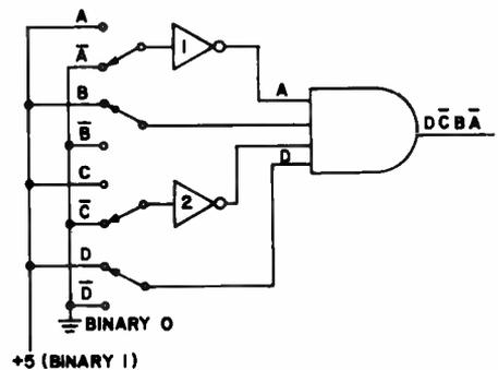
Fig. 6. An AND gate used for decoding the number 1010.
