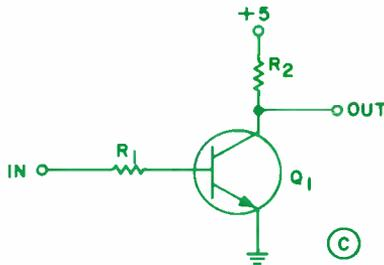
Fig. 2. Inverter symbol (A), truth table for the inverter (B), and a typical inverter circuit (C).
