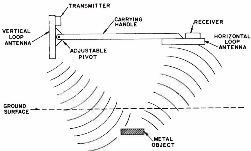
Fig. 1. A typical transmit-receive locater, used for detecting deeply buried objects.
