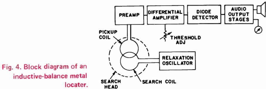
Fig. 4. Block diagram of an inductive-balance metal locator.
