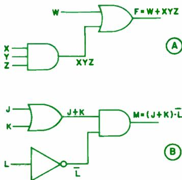
Fig. 5. Two examples of combined logic gates.
