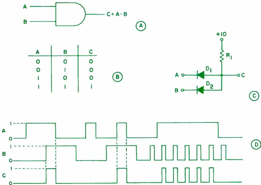
Fig. 3. An AND gate symbol (A), its truth table (B), circuit (C), and input/output waveforms (D).
