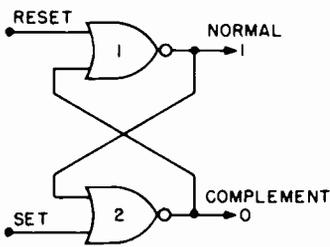
Fig. 2. A NOR gate flip-flop.
