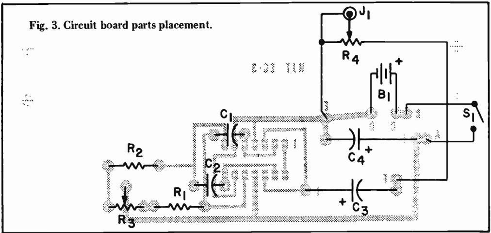
Being careful to install the integrated circuit in the right direction, mount all the components on the circuit board as shown in Fig. 3. The small dimple at one corner of the unit indicates pin #1. Notice that this pin is also identified on the foil side of the board. Of course, all components are to be mounted on the side opposite the foil.
