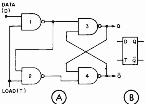
Fig. 4. D flip-flop made with NAND gates (A) and its logic symbol (B).
