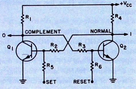
Fig. 1. A simple flip-flop circuit.
