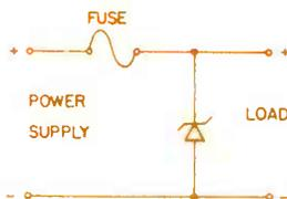
Fig. 7. Zener-fuse combination protects load from excessive supply voltage.
