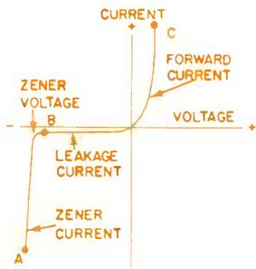
Fig. 1. Relationship between voltage and current in a Zener diode.
