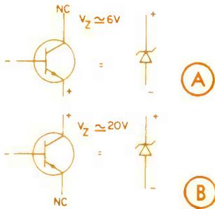
Fig. 8. Substitution of an ordinary transistor for a low-voltage Zener (A), or a high-voltage Zener (B).
