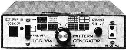
An exciting achievement engineered to meet every service demand, this battery operated, portable instrument offers test patterns of highest quality through digital accuracy. Designed to fit into all tool caddies but practical for shop too. Uses crystal controlled oscillators and flip-flop frequency dividers. Has 8 basic patterns, 2 push button selectable frequencies. Carry case, batteries included.
