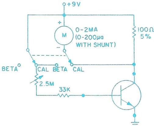
*Fig. 1. Simplified diagram of beta measuring circuit.*
