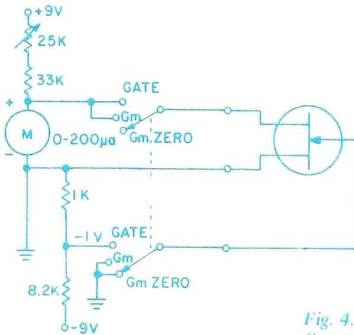
Fig. 4. Simplified diagram of  $G_m$  measuring circuit.
