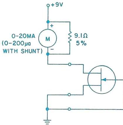
Fig. 3. Simplified diagram of  $I_{DSS}$  measuring circuit.
