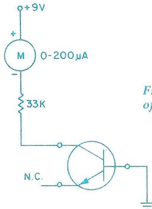
*Fig. 2. Simplified diagram of leakage measuring circuit.*
