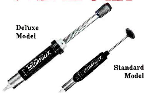
SOLDAPULLT is the best desoldering tool we've seen yet. This tool incorporates easy handling, swift vacuum action and a self cleaning feature. Soldapullt is loaded by pushing plunger knob down until it latches. Molten solder is drawn into its cylinder instantaneously with a high impulsive vacuum by release of the spring loaded piston.
