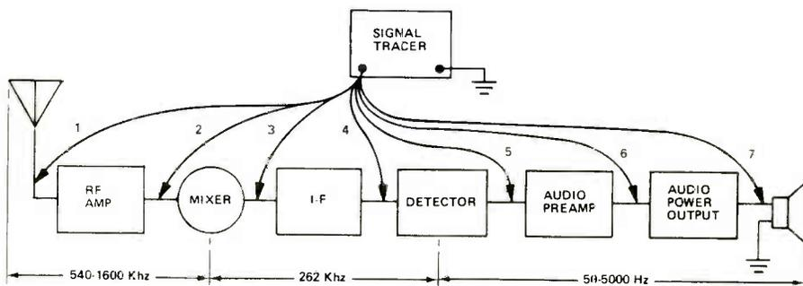
FIGURE 1. SIGNAL TRACING A "DEAD" RADIO.
