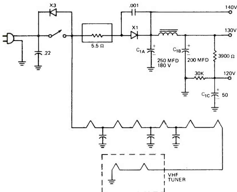
FIGURE 4. LOW VOLTAGE POWER SUPPLY OF ADMIRAL H3-1A. X3 IS FOR INSTANT ON/OFF AND KEEPS THE TUBE FILAMENTS WARM. NOTE ITS POLARITY WITH REGARD TO X1. WITH THE SWITCH OFF, THERE IS NO B-SUPPLY VOLTAGE AND NO REDUCED FILAMENT CURRENT.
