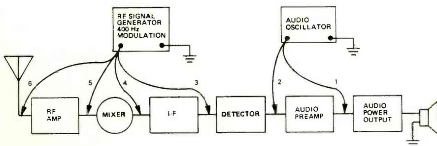
FIGURE 2. SIGNAL INJECTION METHOD OF TROUBLESHOOTING A "DEAD" RADIO.
