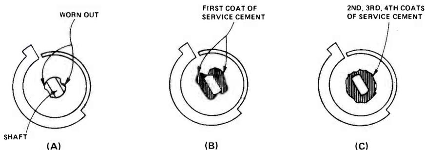
FIGURE 6. WAFER REPAIR.
