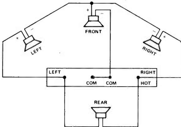
**FIGURE 5. EARLY DYNACO APPROACH FOR REPRODUCING AMBIENT SOUND FROM REGULAR TWO-CHANNEL SOURCES.**
