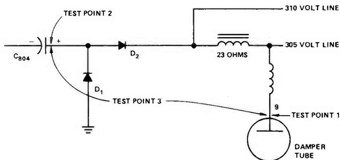
FIGURE 2. SIMPLIFIED SCHEMATIC SHOWING TEST POINTS.
