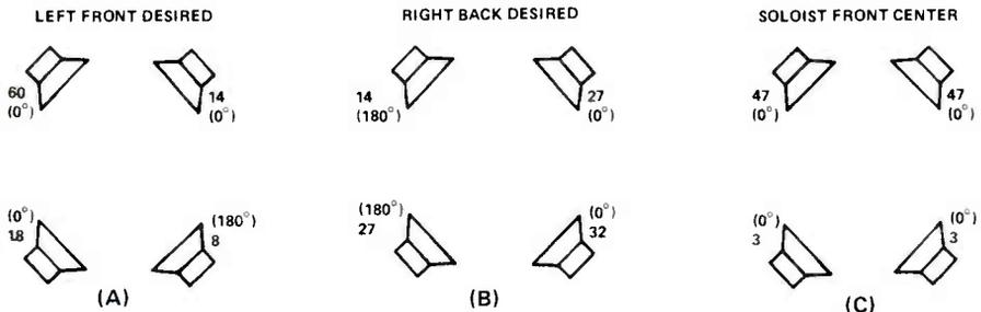
FIGURE 4. POWER AND PHASE DISTRIBUTION FOR THE "OLD" EV DECODER.
