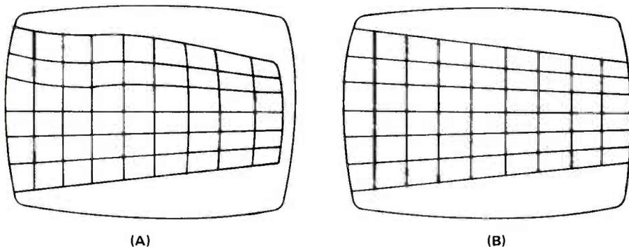
**FIGURE 5. KEYSTONING DUE TO A BROKEN CORE (A) AND DUE TO A SHORTED WINDING (B).**
