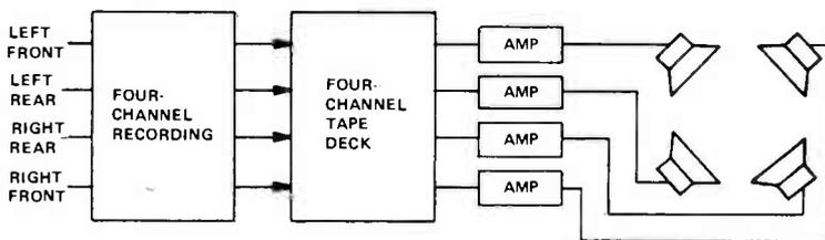
FIGURE 1. DISCRETE FOUR-CHANNEL TAPE SYSTEM.
