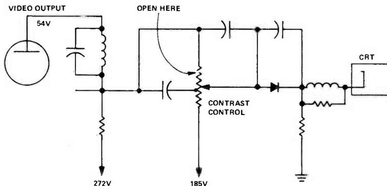
FIGURE 1. SIMPLIFIED SCHEMATIC SHOWING BREAK IN CONTRAST CONTROL.
