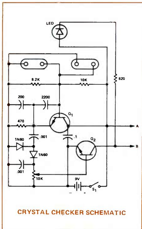
I decided to put in two crystal sockets so that I could plug in either FT-243 or HC-6 type crystals. With the values shown in the schematic, the circuit should oscillate very nicely with crystals from about 1 MHz to 15 or 20 MHz fundamental frequencies. If you go outside of this range you will probably have to play with the values of the emitter resistor and the two capacitors in the base circuit of  $Q_1$ .
