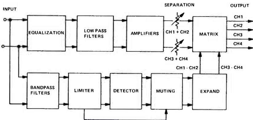
FIGURE 8. CIRCUITRY FOR RECOVERING FOUR CHANNELS FROM DISC.
