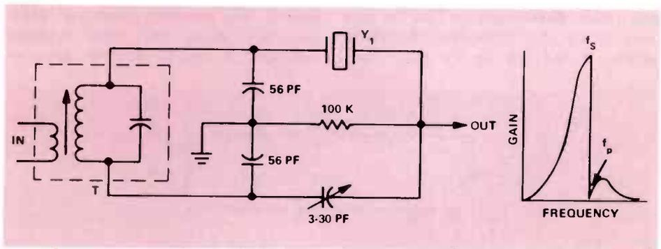
FIGURE 3. CW FILTER AND RESPONSE.
