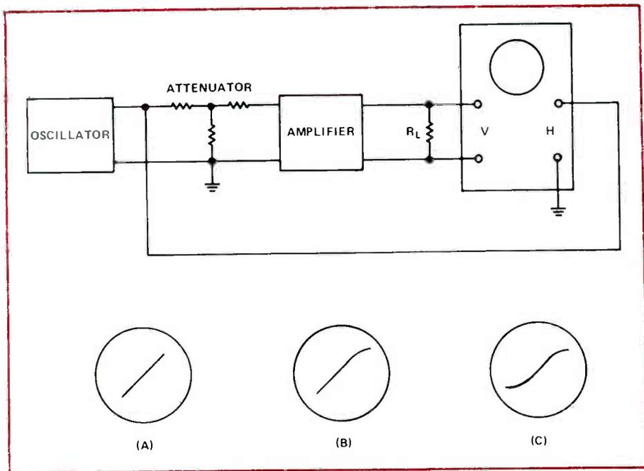
FIGURE 3. OBSERVING HARMONIC DISTORTION USING AN OSCILLOSCOPE.
