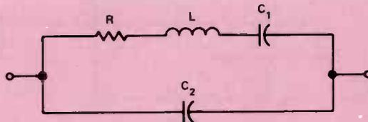
FIGURE 1. ELECTRICAL EQUIVALENT OF A QUARTZ CRYSTAL.
