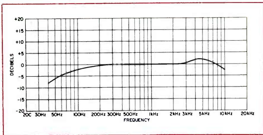
FIGURE 5. AMPLIFIER FREQUENCY RESPONSE.
