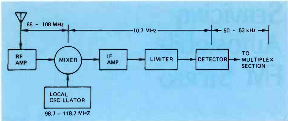
**FIGURE 1. BLOCK DIAGRAM OF A TYPICAL FM SECTION.**
