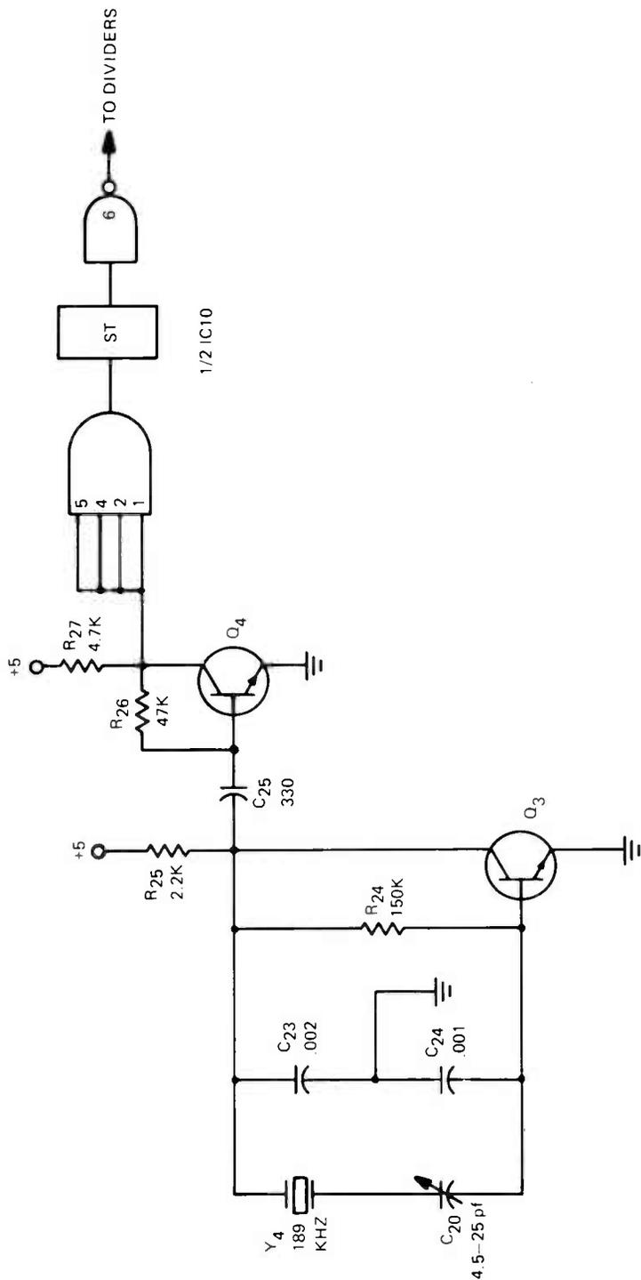
FIGURE 5. SCHEMATIC DIAGRAM OF CLOCK AND SHAPER.
