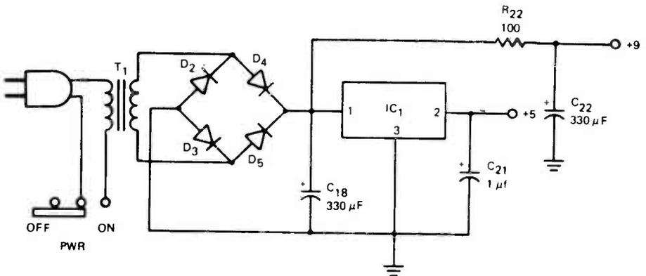
FIGURE 4. SCHEMATIC DIAGRAM OF THE POWER SUPPLY.
