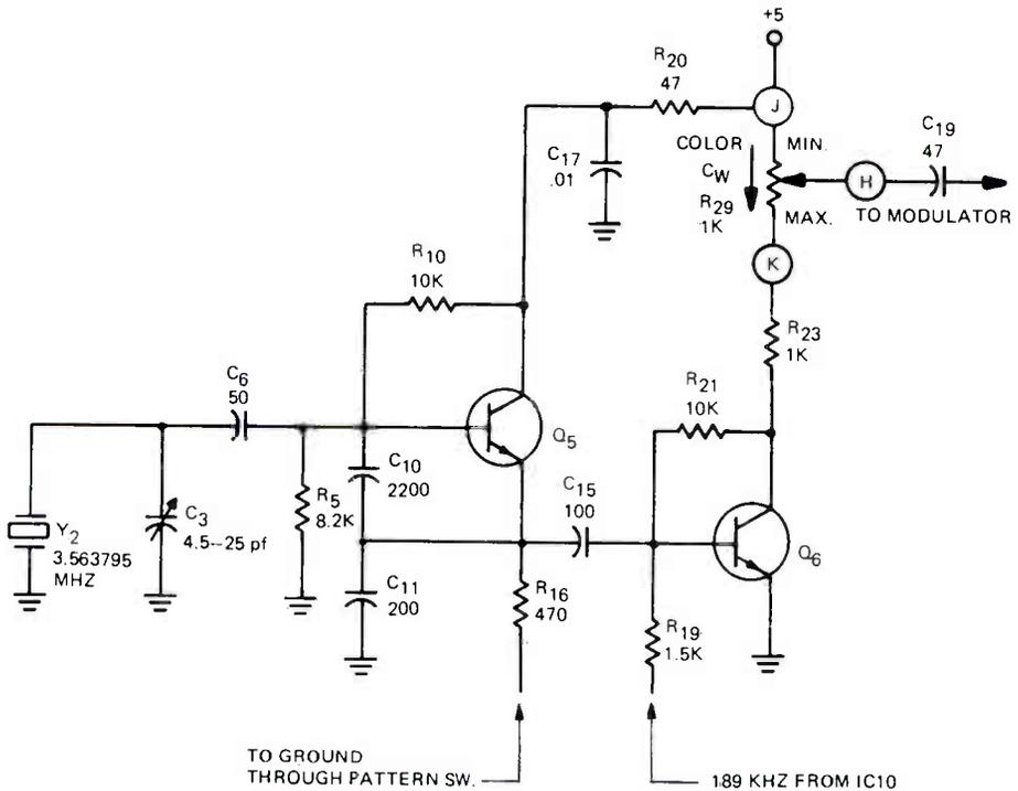
FIGURE 9. SCHEMATIC DIAGRAM OF THE COLOR OSCILLATOR AND SWITCH.
