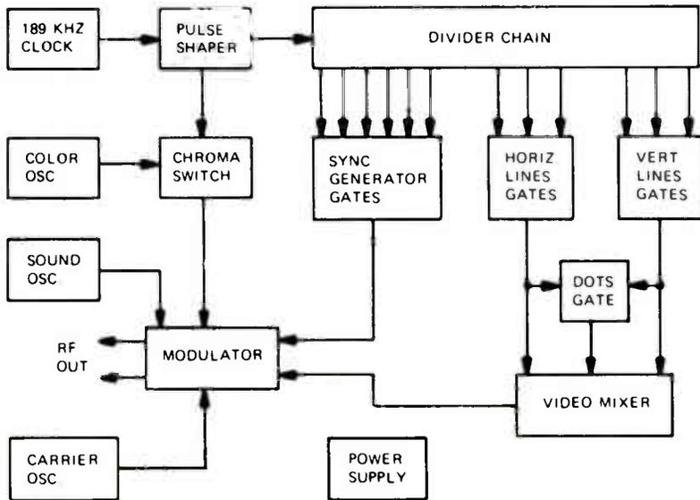
FIGURE 3. SIMPLIFIED BLOCK DIAGRAM OF THE TV PATTERN GENERATOR.
