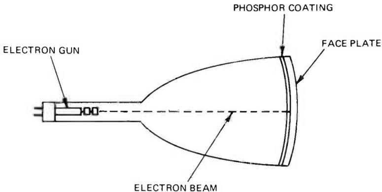
FIGURE 2. SIMPLIFIED DRAWING OF A TELEVISION PICTURE TUBE.
