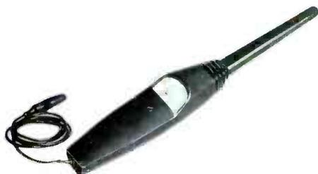
For fast, accurate, safe high-voltage measurements up to 30,000 volts. Extremely lightweight for ease in handling, yet very rugged. Built-in overload capability. Tracking accuracy,  $\pm 2\%$  of full scale. Reading accuracy, 2% at 25 KV. Meter movement includes self-shielded bar magnet. Housing is anti-static treated. Knife-edge pointer and large numbers for ease of reading. 1.75" probe tip for reaching under corona cap. Shpg. wt., 1 1/2 lbs.
