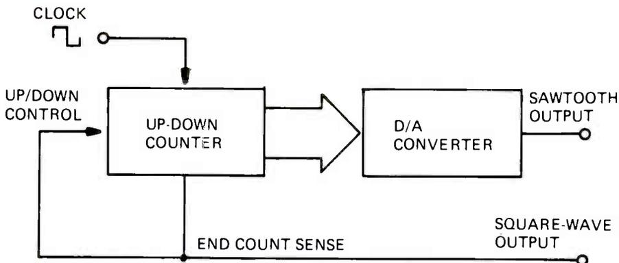
FIGURE 5. BASIC DIGITAL FUNCTION GENERATOR.
