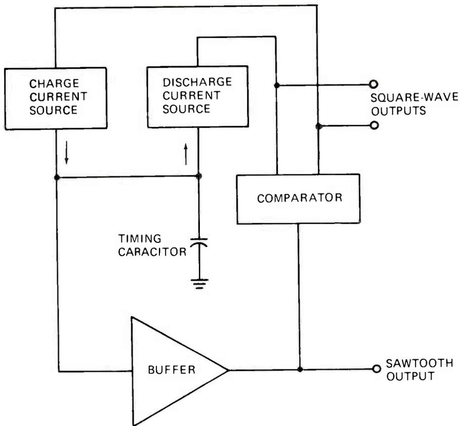
FIGURE 2. THE HEART OF THE FUNCTION GENERATOR.
