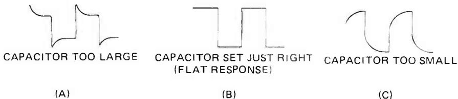
**FIGURE 3. WAVEFORMS WITH VARIOUS CAPACITOR SETTINGS.**
