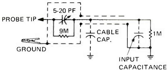
**FIGURE 2. BASIC 10:1 LOW-CAPACITANCE PROBE. ADJUSTABLE CAPACITOR IN PROBE IS SET FOR FLAT RESPONSE.**
