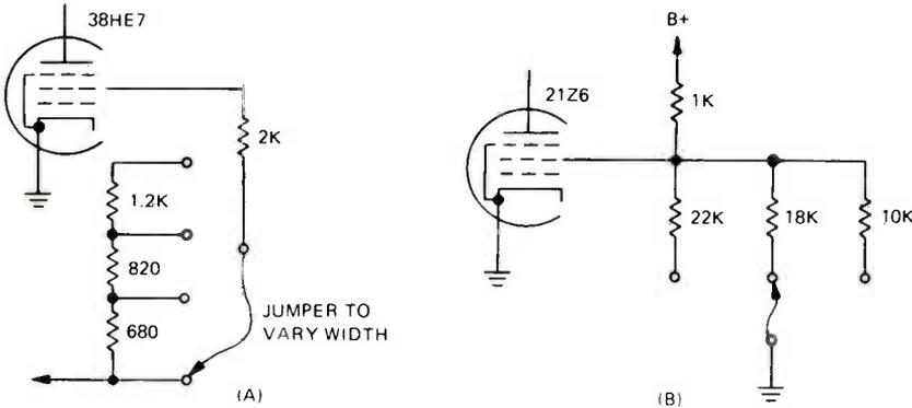
FIGURE 3. WIDTH ADJUSTMENT USING SERIES (A) AND SHUNT (B) RESISTOR.
