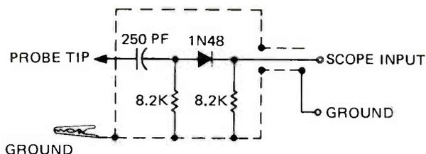
FIGURE 6. A DEMODULATOR PROBE.
